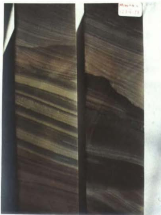
Plate 3.3: Very fine-grained sandstone and siltstone with erosional surfaces and low-angle cross-lamination, Rodda beds correlative, 1233.0 m, 1234.7 m depths, Munta 1 drillhole, Officer Basin. Core is 60 mm diameter.
