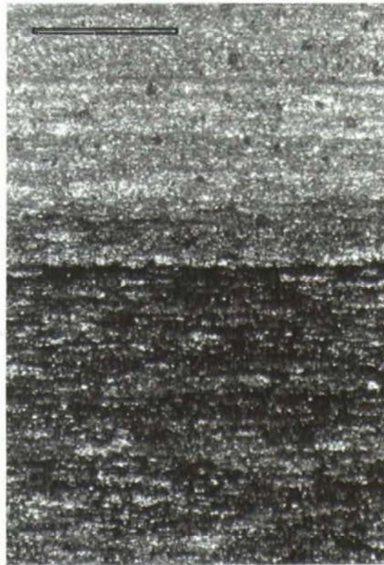
Plate 2.2: Thin section, mudstone with thin, anastomosing, organic-rich laminae (benthic microbial mats) overlain by organic-poor mudstone with planar-parallel lamination. Pertatataka Formation, sample 28.112, 1206.5 m depth, Wallara-1 drillhole, Amadeus Basin. Scale bar = 1mm.
