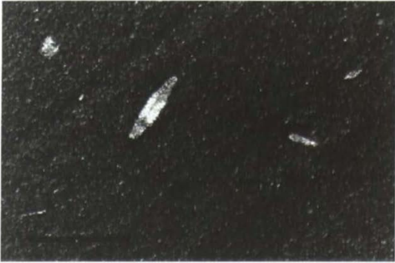
Plate 3.4: Lenticular gypsum crystals in calcareous mudstone, sample 5.43, Unit 5, Wonoka Formation, Bunyerroo Gorge. Scale bar = 1mm.
