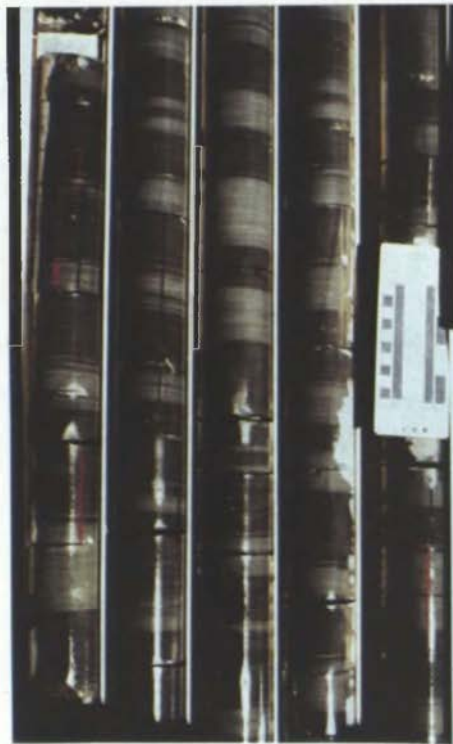
Plate 4.5: Drillcore showing interbedded black shale (benthic microbial mat facies) and grey-green shale in lower part of Pertatataka Formation, 1236-1241 m depth, Wallara 1 drillhole. Core is 60 mm diameter.
