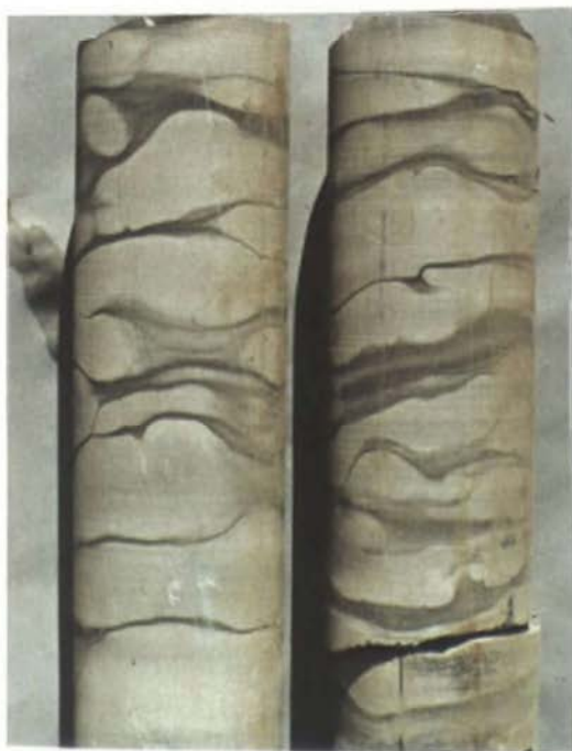
Plate 3.2: Nodular bedding in micritic limestone. 'Karlaya Limestone' unit of Rodda beds correlative, 1661 m depth, Munta 1 drillhole, Officer Basin. Core is 60 mm diameter.
