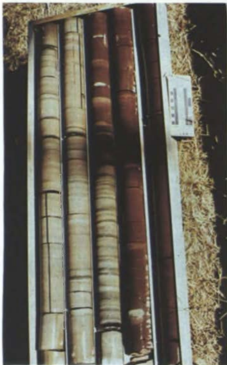
Plate 4.4: Drillcore showing upward gradation from pale buff-coloured, laminated 'cap dolostone' into massive red mudstone of the basal Pertatataka Formation. Note diffuse nodules and layers of dolostone in basal part of red mudstone. Wallara 1 drillhole. Core is 60 mm diameter.
