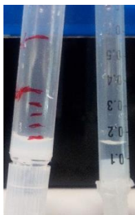
Figure 1. Photo of resin bound B4GALT1 packed onto a column (left) and a syringe (right). 100 \mu l of bed volume was estimated by markings made using known volumes. The inner diameter of the syringe (bed dimension ~ 4mm diameter X 5mm height) is approximately half that of the column (bed dimension ~ 7mm diameter X 2mm height), resulting in a longer resin bed. The measured flow rate, assisted by capillary action (i.e. tip of column and syringe was in contact with the walls of the collection tube) was approximately 40s/ml for the column and 100s/ml for the syringe.
