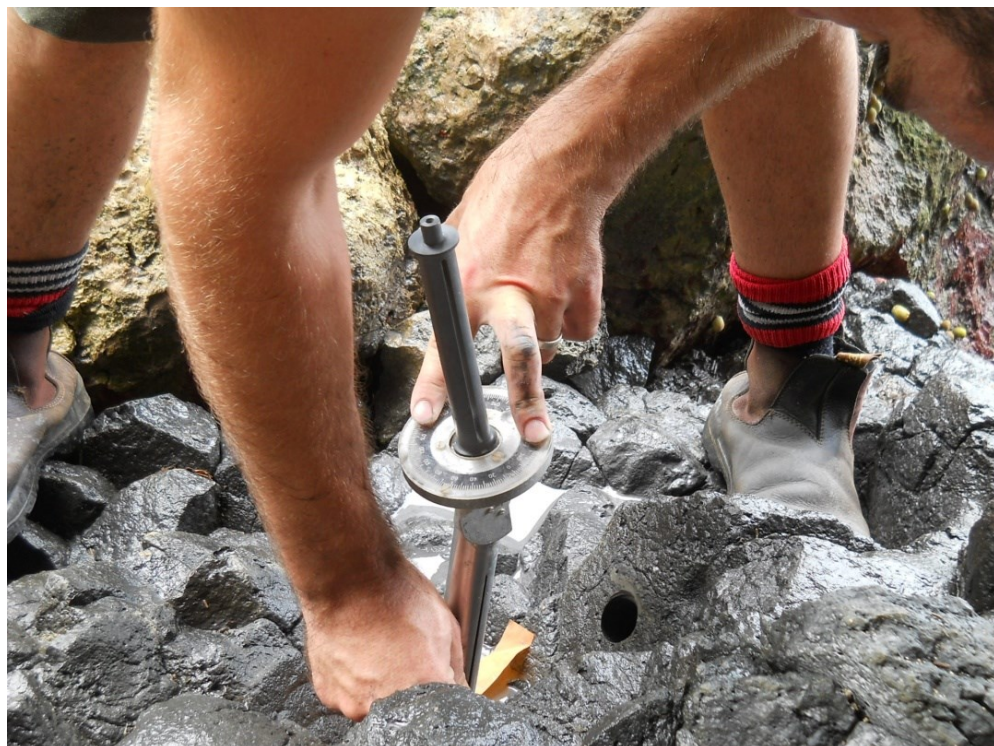
Figure 3.3: Orientation of a sun compass while taking drilled core samples for paleomagnetic interpretation at Waterfall Spring. Dr. Craig O'Neill measuring the orientation of the drilled core.
