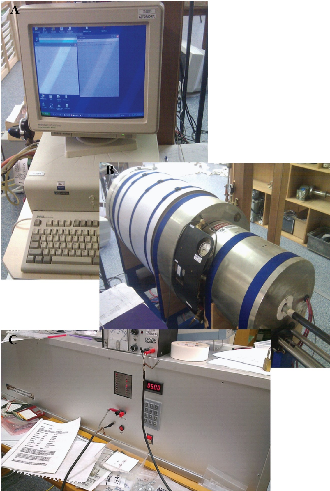
Figure 3.10: Paleomagnetic laboratory setup at CSIRO (North Ryde) showing the computer (A), operating the AF-demagnetiser (Model 2G600) (B), and the thermal demag (MMTD80) furnace (C) at temp 500° C. For AF-Demagnetisation, drilled sample is put in the long black tube at one end of the AF-demagnetiser, while the computer reads the values. For thermal demagnetisation, samples are first thermally heated in the furnace (C) and then the value is read in the AF-Demagnetisation machine (B).
