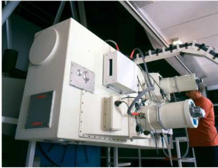
FIGURE 2.1: A picture of the DBS, mounted on the 2.3 Metre telescope. The blue arm is to the left and the red is to the right.
