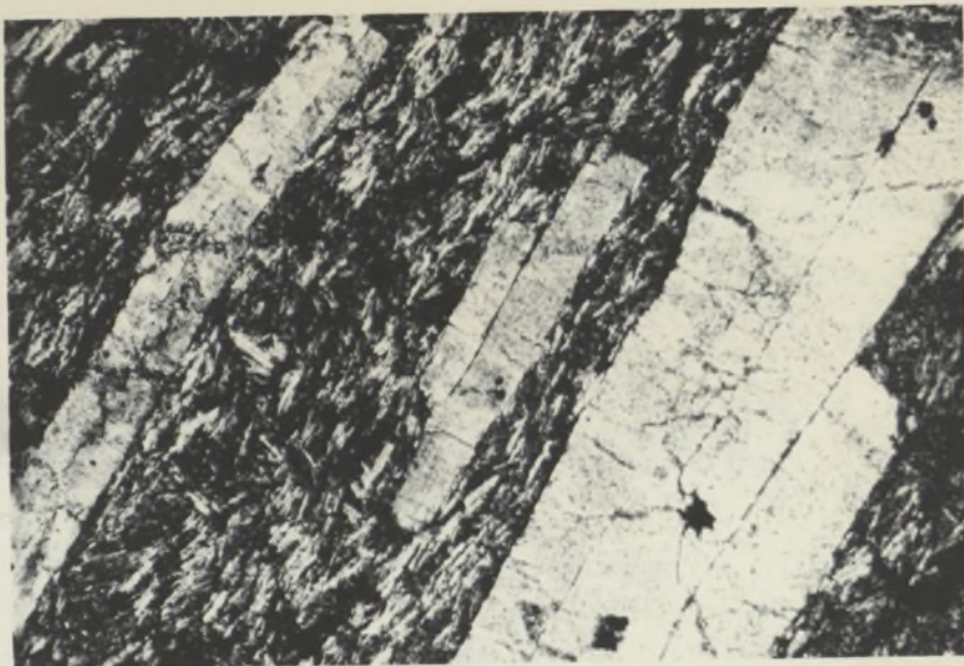
Albitised(?) relict plagioclase phenocrysts in metabasalt. (S.N. 287), C.N., x 100
