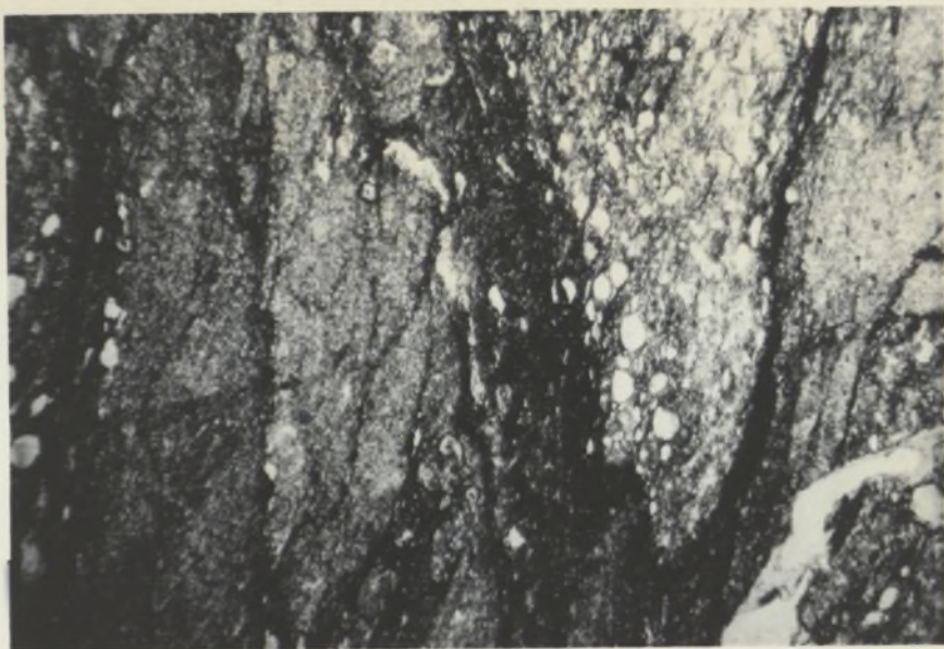
Radiolaria and quartz rich patches in deformed pelitic rock (S.N. 180) P.P., x 130
