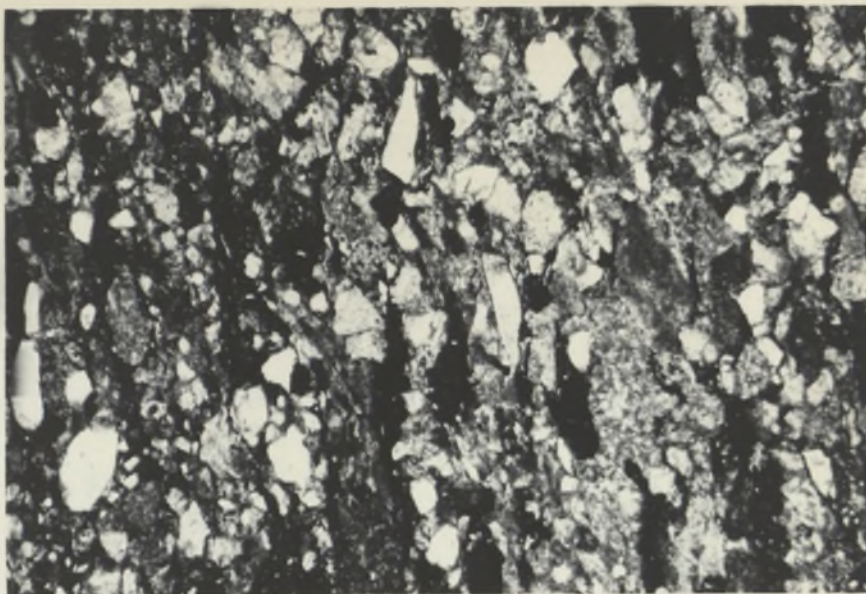
Unmetamorphosed lithic sandstone showing rock and mineral fragments in fine matrix. (S.N. 146), P.P., x 100
