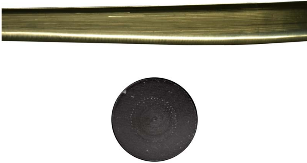
Figure 53: Picture of the TOPAS fiber cane after the second draw run (fabricated at DTU).
