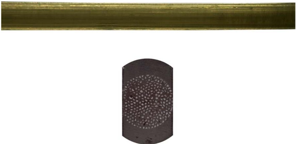
Figure 51: Photograph of the PC THz filter drawn preform and a cross section of the design fabricated at USYD.
