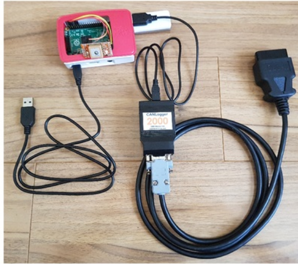
Figure 4.1: The Electronic Vehicle Monitoring System
