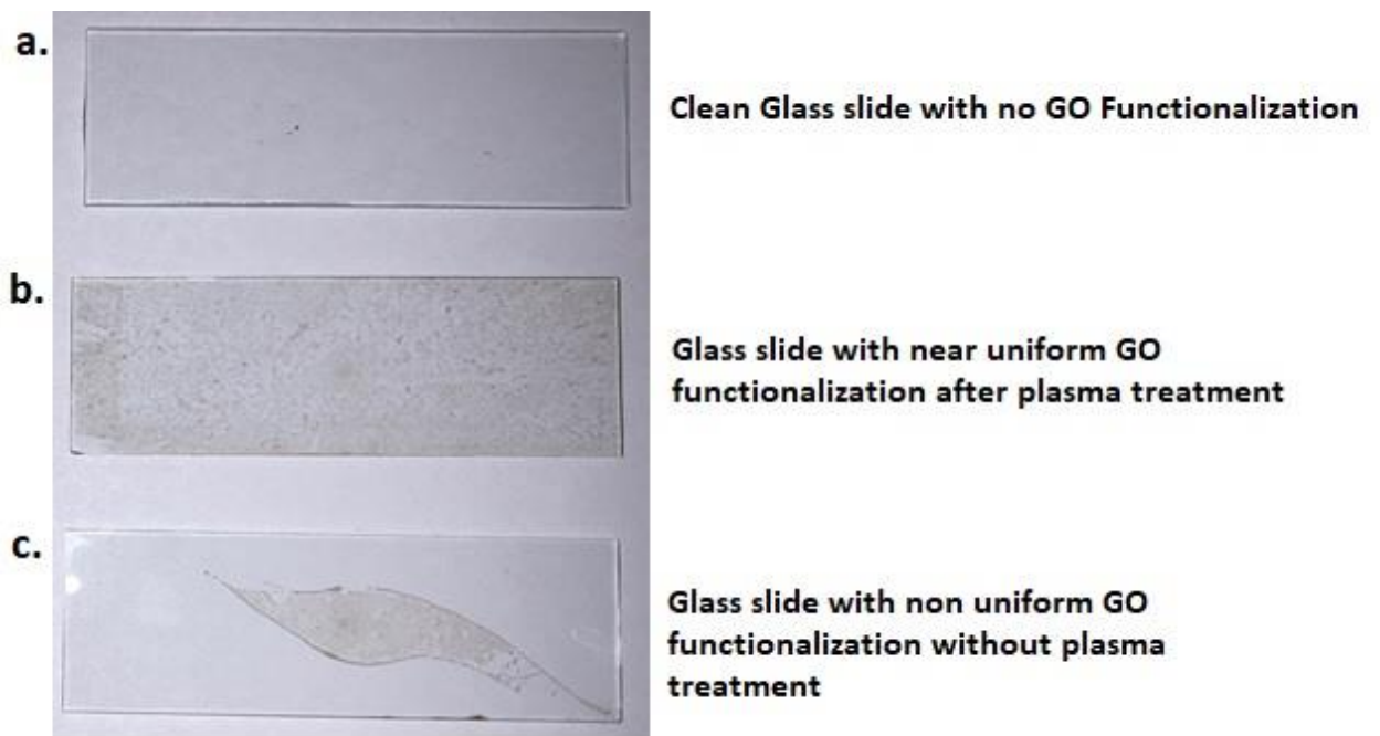
Figure 14. Images of Glass slides with and without oxygen plasma treatment before GO coating
