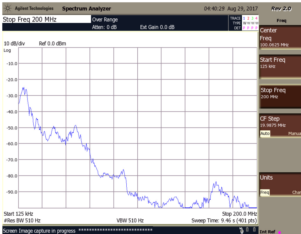
Figure 5.20. Spectrum of conducted EMI for a) simple SPWM (125 kHz ~ 100 MHz), b) aperiodic SPWM (125 kHz ~ 100 MHz), c) simple SPWM (125 kHz ~ 200 MHz) and d) aperiodic SPWM (125 kHz ~ 200 MHz).
