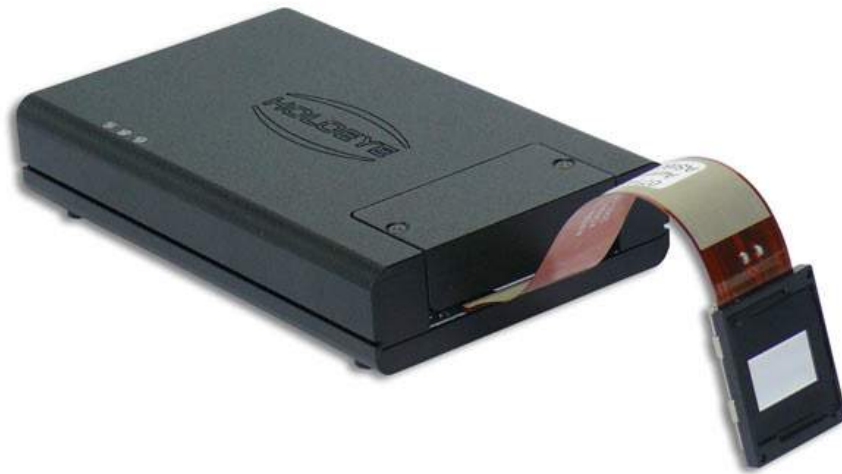
Figure 3.3: Spatial Light Modulator. Producer: Holoeye photonics AG . Model: PLUTO-NIR-015-HR . The active area is limited to the mirror-looking rectangle in the bottom-right part of the photo. The black plastic box in the back encloses the driver unit. Source: http://holoeye.com/spatial-light-modulators/slm-pluto-phase-only/
