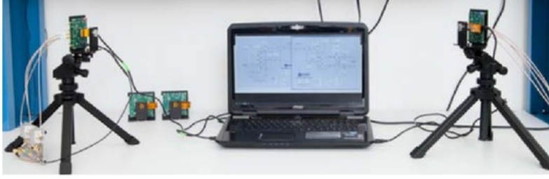
Figure 5.1: Pasternack 60GHz Development System
