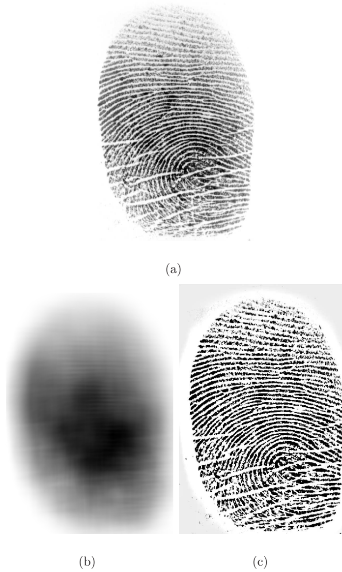
Figure 3.10: Background homogenization process: Fig. (a) shows an acquired digital fingerprint. Fig. (b) depicts the estimated non-uniform background. Fig. (c) is an output result after passing the image through homogenization operation and then linearly stretched. It can be observed that contrast has been corrected with clear ridge/valley structure.
