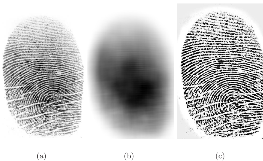
Figure 4.11: Non-uniform illumination correction. a) shows an acquired digital fingerprint. b) depicts the estimated illumination surface, clearly showing non-uniform background lighting conditions. c) is an output result after passing the image through homomorphic filtering operation and then linearly stretched. We observe that illumination has been corrected with clear ridge/valley structure
