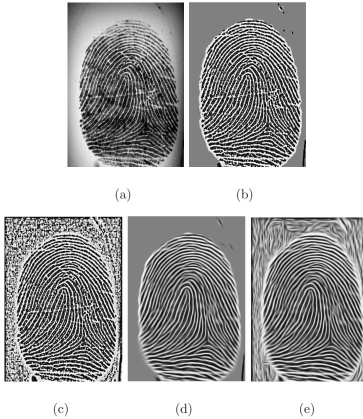
Figure 6.6: The impact of diffusion process on normalisation: a) Sample image. b) Image normalised with factor. c) Image normalised without factor. d) Diffused image after normalising with factor. e) Diffused image after normalising without factor.
