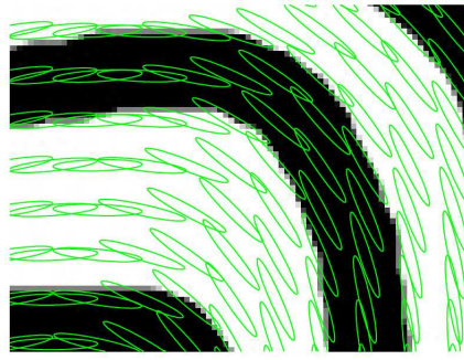
Figure 4.7: Geometric interpretation of diffusion matrix. The figure shows part of the anisotropic curve image. The diffusion matrix associated with each pixel is depicted as ellipses on top of the image. It is observed that ellipses are steered to follow with the curve flow direction
