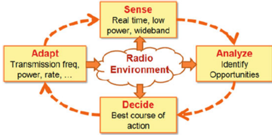
Figure 2.1: Functional Architecture of a Cognitive Radio
