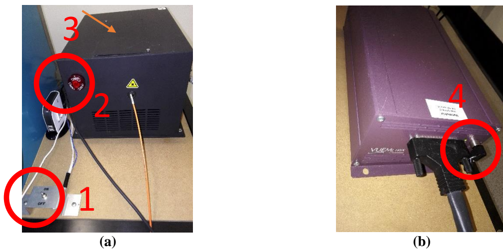
Figure 3.5. A 30 W Helight Raylas laser (a) with its VueMetrix Vue-HCT Controller (b). The laser is provided with four interlocks: a bench top on/off switch (a.1), an emergency push button switch (a.2), a failsafe door interlock (a.3), and an interlock key switch on the controller (b.4).
