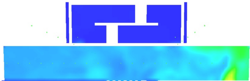
Figure 5.29: Temperature at 2m above floor level on the floor of fire origin at 300 seconds.
