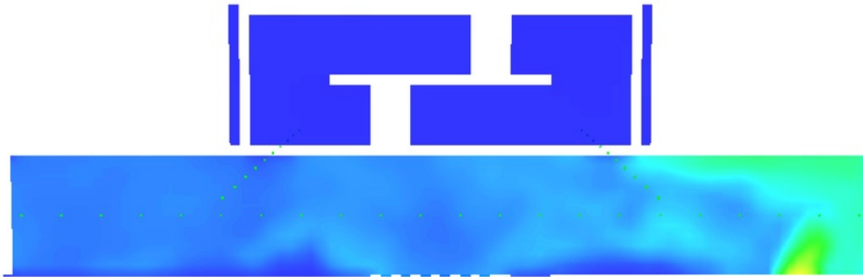
Figure 5.7: Temperature at 2m above floor level on the level of interest with 2 doors open.
