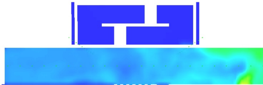
Figure 5.12: Temperature at 2m above floor level on the level of interest with 4 doors open.
