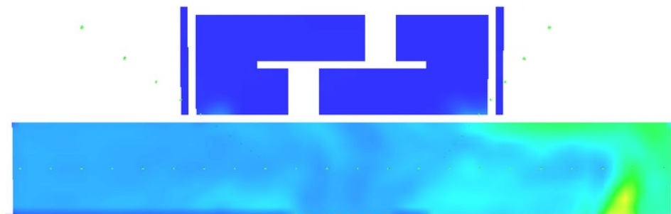
Figure 5.17: Temperature at 2m above floor level on the level of interest with 6 doors open.
