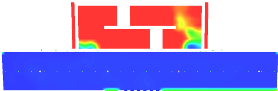
Figure 5.15: Visibility at time t = 300 , with 6 doors open
