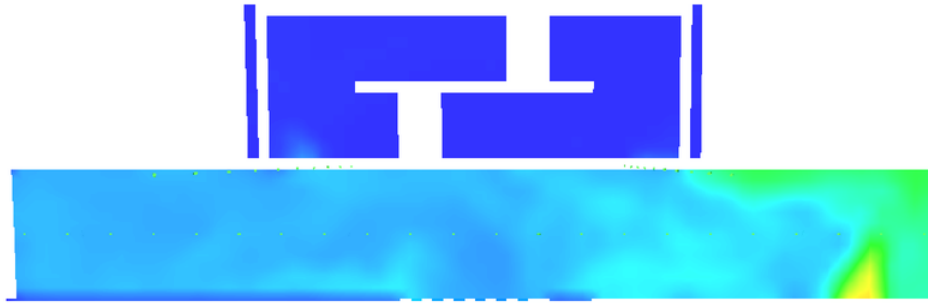
Figure 5.23: Temperature at 2m above floor level on the level of interest with 8 doors open.
