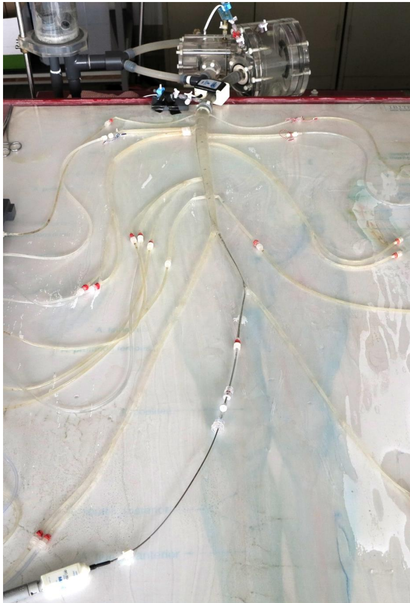
Figure 5.1: Picture of the whole silicon distributed model of the arterial circulation, connected to the pumping system (top). The flow probe is placed around the ascending aorta and the Millar catheter is inserted via a dedicated inlet at the left common iliac artery.
