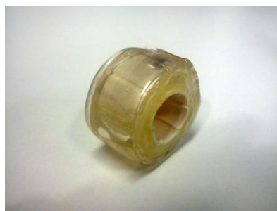
Figure 4.2: “Plug” connector composed of a rigid cylindrical core and several external layers of Tygon sealed with silicon glue and hot glue.
