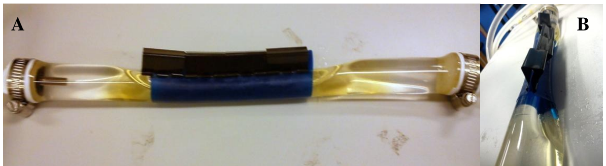
Figure 4.7: Beginning of experiment with a single rectangular wrap derived from a physiotherapy elastic band. A) Wrapped silicon aortic model at zero pressure; B) detail of the wrap.
