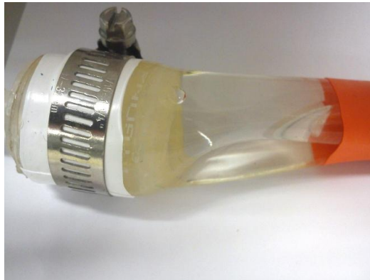
Figure 4.17: Detail of the folded shape that the silicon aortic model assumed after wrapping.
