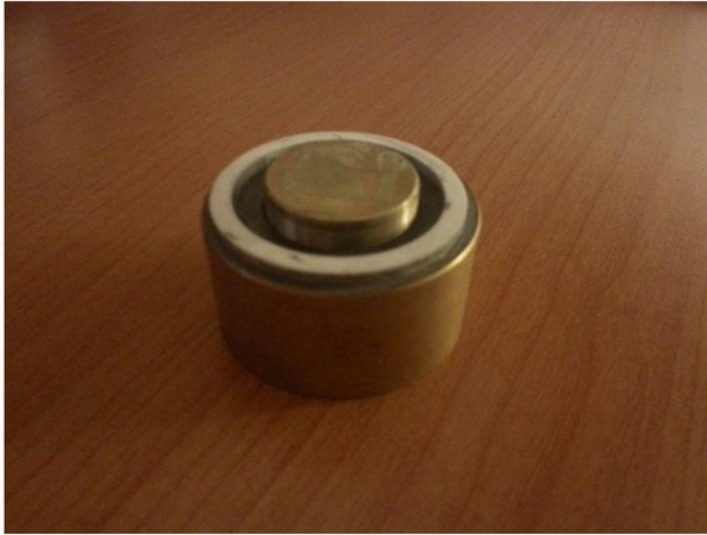
Figure 4 - Brass and ceramic sanding device used to assist sanding
