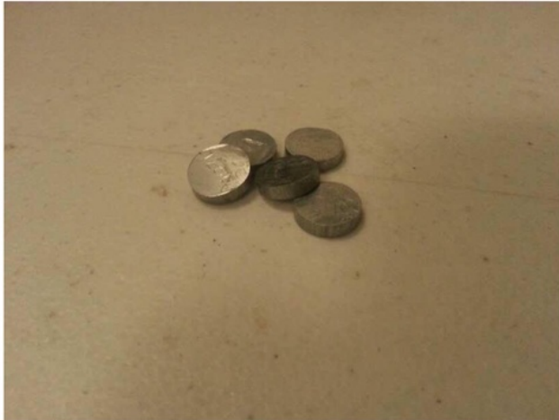
Figure 3 - Zinc samples cut using Struers ACCUTOM cutting machine
