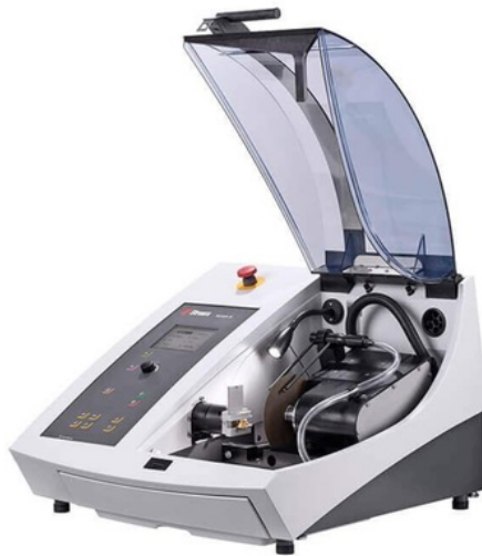
Figure 2 - Struers ACCUTOM cutting machine
