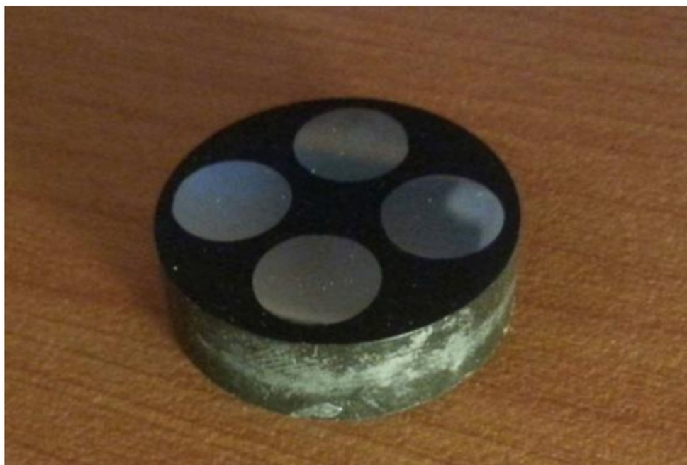
Figure 6 - 4 pieces of zinc mounted using mounting press
