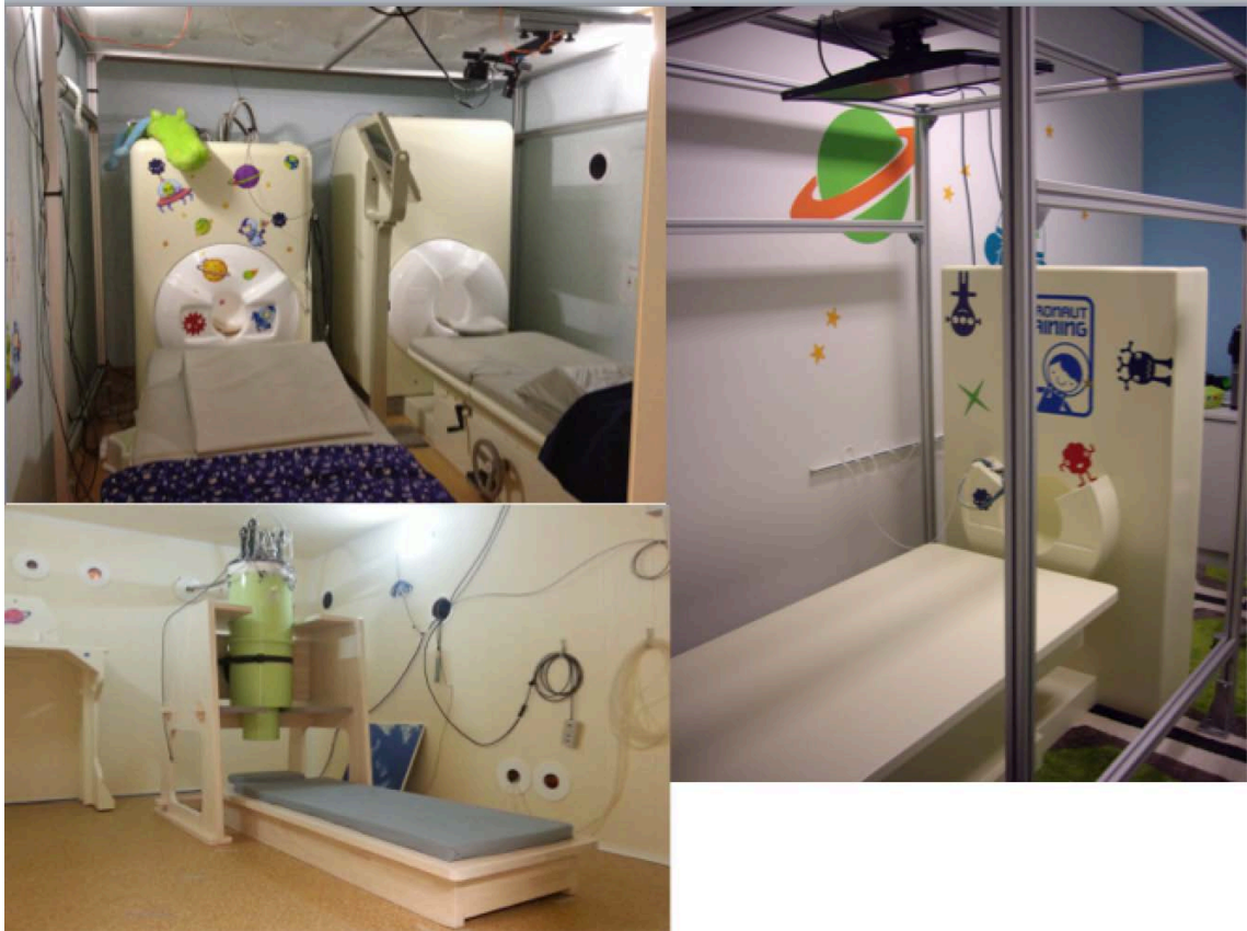
Figure 1: MEG systems at the KIT-Macquarie Brain Research Laboratory located at the Australian Hearing Hub, Macquarie University. Top left. Adult (right) and child (left) MEG systems are located side by side within a single magnetically-shielded room. The adult MEG has 160 SQUID sensors, the child system has 125. Both systems are designed for supine positioning of participants. The child system is sized for preschool children aged 3-5 years. Right. MEG simulator for training of child participants. Bottom left. Prototype MEG system engineered for use with unilateral cochlear implant recipients.
