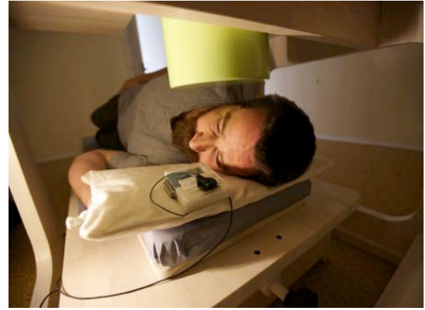
Figure 21: The custom-engineered MEG system for cochlear implant recipients. Left: Appearance of the system. Right: Demonstration of the experimental setup with a normal hearing person and a CI emulator box by the side of his head (figure for display only, during the actual experiment MEG sensor plane touched the side of participant's head and the CI emulator was placed underneath the other side of the head).
