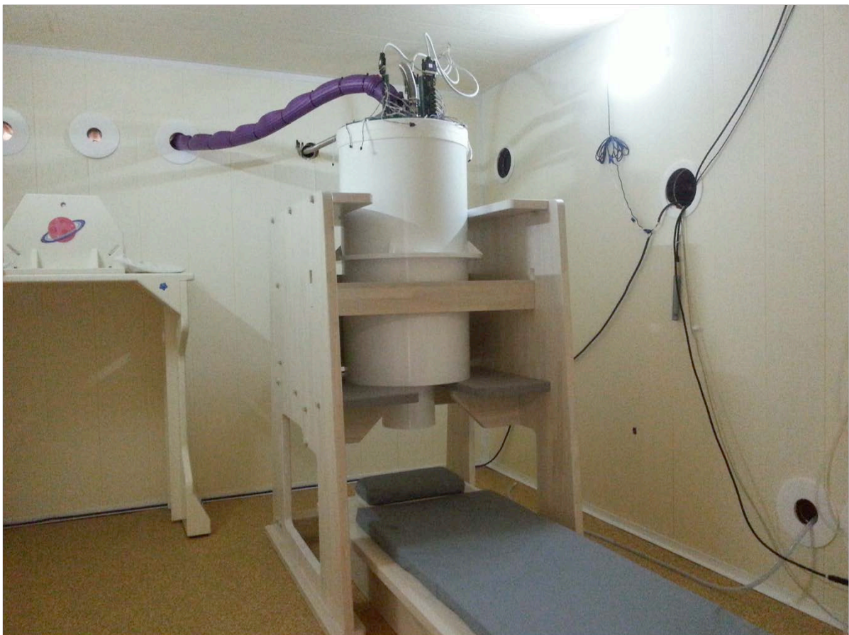
Figure 26: The upgraded MEG system with two types of irregular baseline second-order gradiometers
