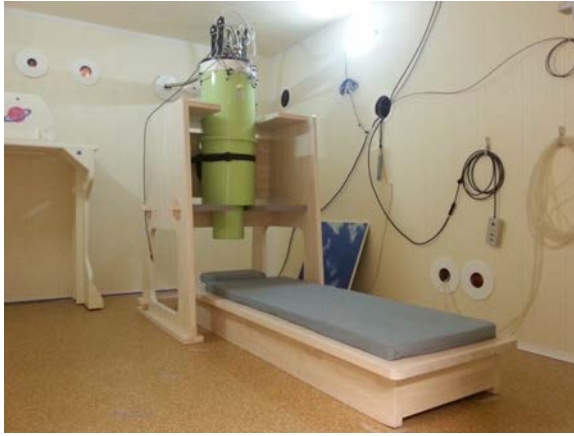
Figure 21: The custom-engineered MEG system for cochlear implant recipients. Left: Appearance of the system. Right: Demonstration of the experimental setup with a normal hearing person and a CI emulator box by the side of his head (figure for display only, during the actual experiment MEG sensor plane touched the side of participant's head and the CI emulator was placed underneath the other side of the head).
