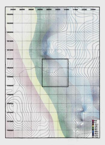
Figure 7.4 Bouguer Gravity map covering the Manilla area. The square shows half-circle gravity low indicating a possibly low density granite beneath.
