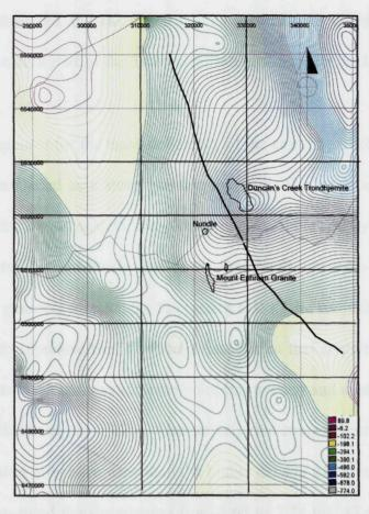
Figure 7.5e. Bouguer gravity map covering the Nundle area. The thick black line shows the location of the Peel Fault. The gravity low corresponding to the Duncans Creek Trondhjemite and Mount Ephraim Granite indicates a possibly large low-density pluton beneath.
