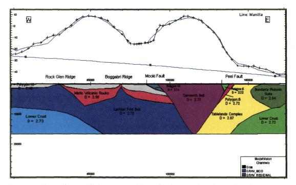
Figure 7.9a 2D gravity model along the Manilla Profile (cross-section view). The reflection seismic model by Korsch et al. (1997) was used to constrain the subsurface geometry of the structural units along the Manilla profile. Polygons 5, 6 represent the high density Woolomin Association, 10 the Gunnedah Basin, and 13 the Tamworth belt Between the Mooki and Kelvin Faults.
