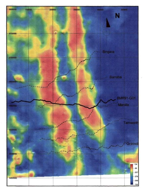
Figure 7.1 The location of the gravity profiles surveyed in this study, shown on the regional Bouguer gravity map. From south to north, the gravity profiles are named Quirindi, Tamworth, Manilla, Barraba and Bingara. The profiles are approximately normal to the north-north-west trending Meandarra Gravity Ridge to the west and Namoi Gravity High to the east. Also shown is the position of the deep reflection seismic line BMR91-G01.
