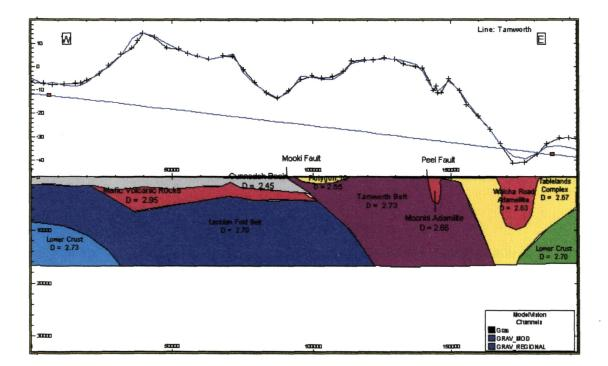
Figure 7.10 2D gravity model along the Tamworth Profile (cross-section view). The Peel Fault was modelled as a shallow east-dipping fault with a low density Woolomin Association. Polygon 10 represents the Werrie Basin. Symbols represent observed data and solid line is the calculated anomaly, V/H=2. Density in tm<sup>-3</sup>, scale in metre.
