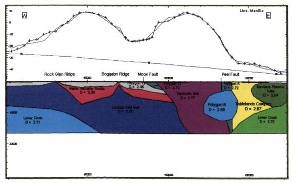
Figure 7.9b 2D gravity model along the Manilla Profile (cross-section view). The Peel Fault was modelled as an east-dipping fault with a depth extent of 15 km. Polygon 4 represents the high density Woolomin Association, 6 a low density unit, 13 the Tamworth belt Between the Mooki and Kelvin Faults and 12 the Gunnedah Basin. Symbols represent observed data and solid line is the calculated anomaly, V/H=2. Density in tm<sup>-3</sup>, scale in metre.
