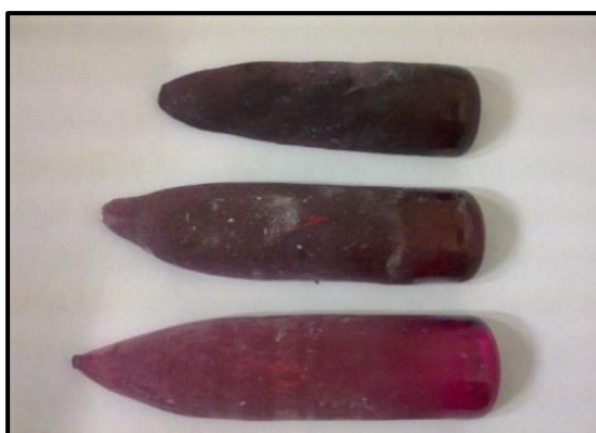
Figure 2.1 Three types of synthetic ruby crystals with different chromium concentrations: (a) Sample 1 (Dark rose), (b) Sample 2 (Rose) and (c) Sample 3 (Pink rose)
