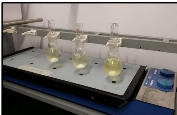
Figure 6.4 Stirring silver with ammonium hydroxide and TEOS on a multipoint stirring plate for 24 hours to make silica-coated silver nanoparticles
