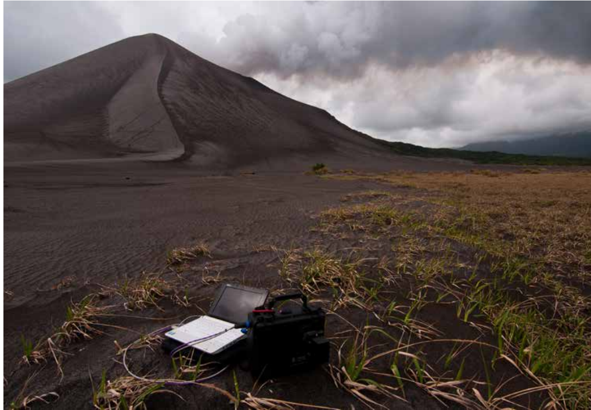
Fig. A1.1 The SO 2 monitoring set-up employed at Yasur during a stationary scan on the ash plain. Note the small size of the Flyspec, which is entirely housed within the black case in the centre of the image, and is connected to a small notebook computer for data capture. The gas plume from Yasur is obvious in the upper right of the image.
