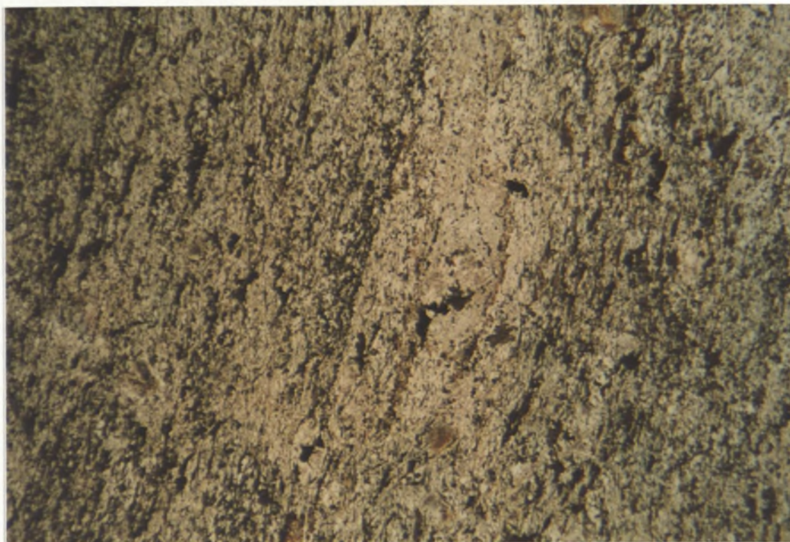
Plate 26. Tw 193. Biotite-quartz assemblage in the lower hornblende hornfels facies. The biotite is platy and is orientated along bedding. (PPL 1·25)
