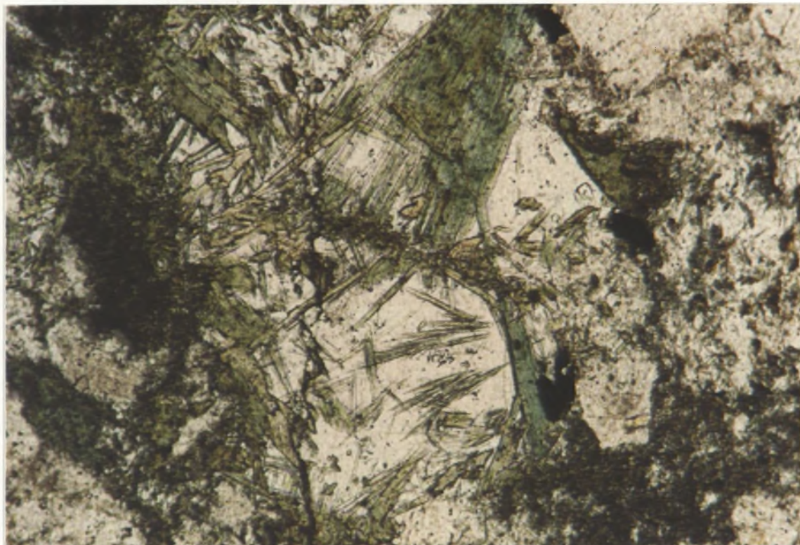
Plate 30. Tw 177. Blue-green fibrous amphibole in albite-epidote hornfels facies. (PPL 6·3)
