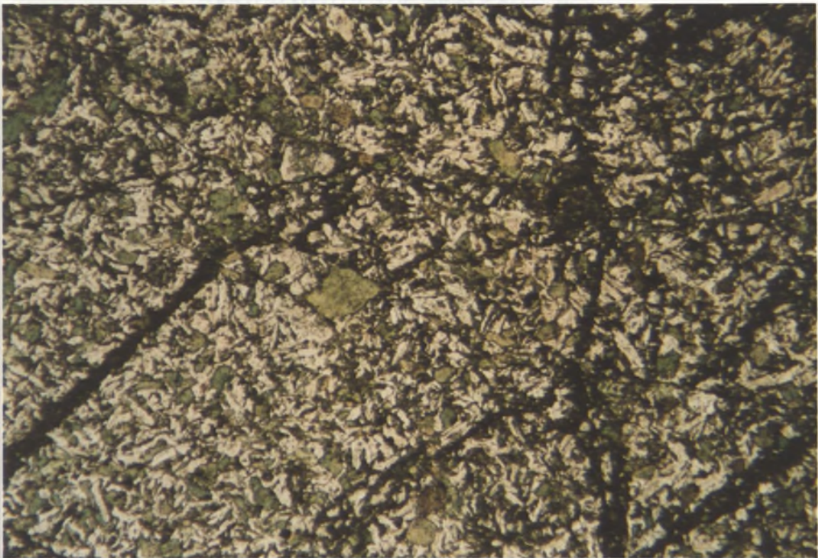
Plate 11. Tw 147. Dolerite. Plagioclase grains do not show alignment as Tw 176. (PPL 1·25)
