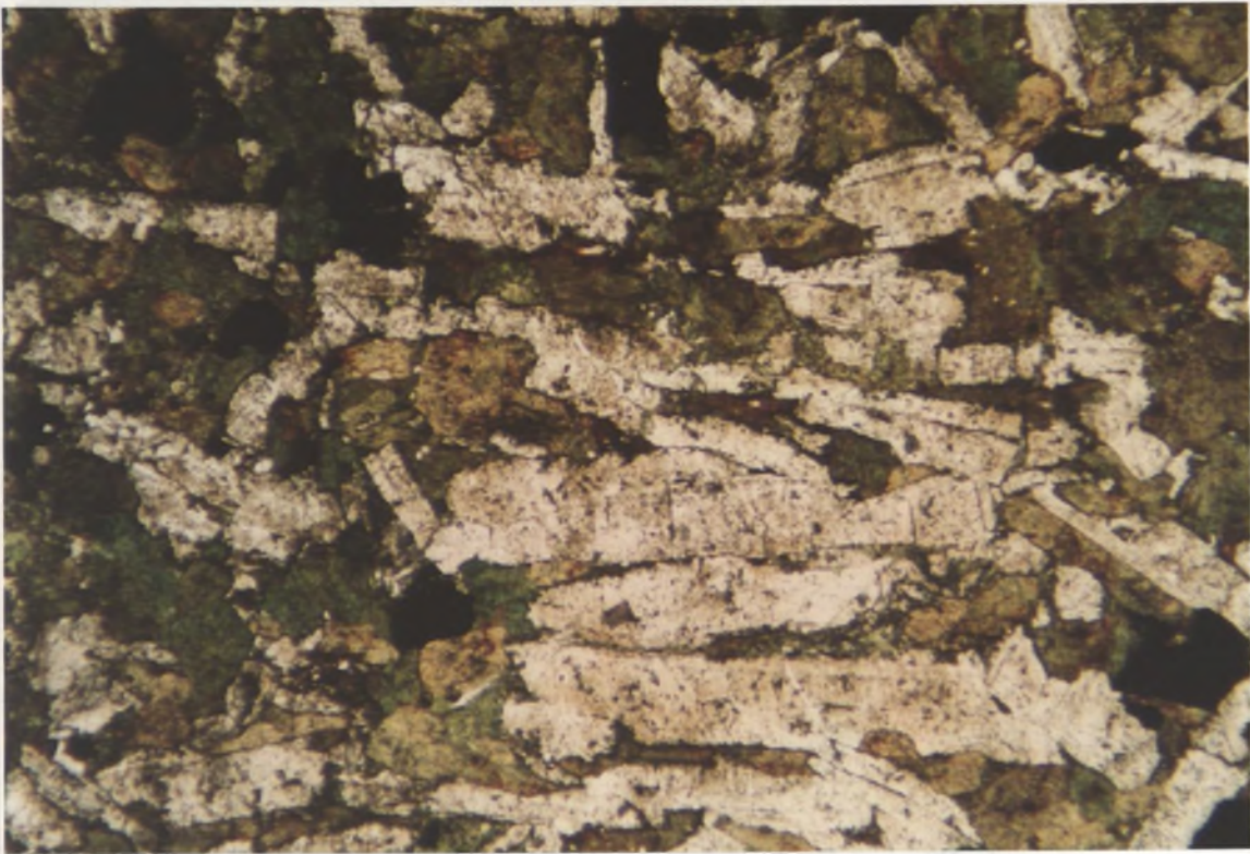
Plate 10. Tw 176. Dolerite from southern area. Green-brown hornblende and aligned plagioclase grains. (PPL 6·25)
