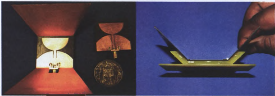
Figure 4.24: Hardware prototype of CPW-fed semicircular-disc monopole antenna with the surface integrated short TEM horn.
