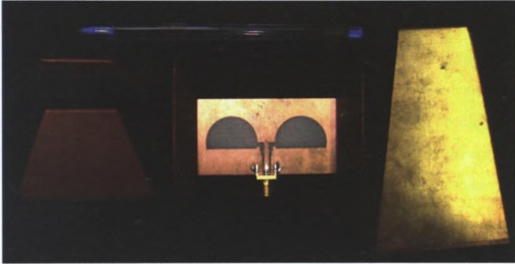
Figure 6.17: Hardware prototype of PSSA with integrated horn and various other short horns of different length.
