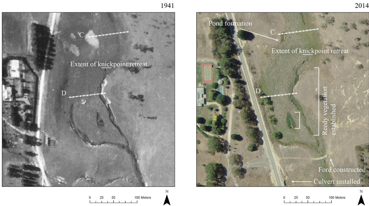
Figure 3.10: The knickpoint shown here remains active and has retreated approximately 30 m since 1941. Some stabilisation of sediments downstream of the knickpoint has also taken place with the appearance of reed beds.
