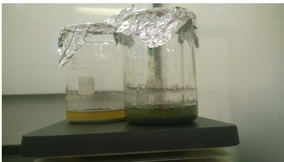
Figure 3.1.3. AK005 and AK019 samples on a hot plate after addition of 6% HCL.
