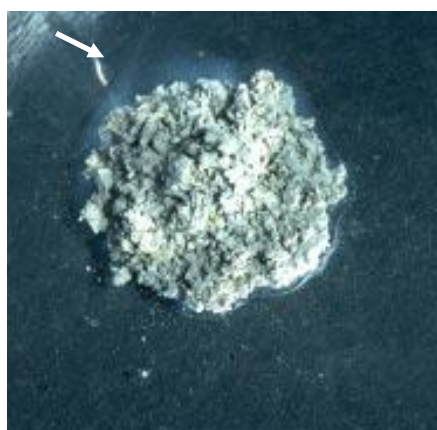
Figure 14: Slaking of a soil aggregate. Slight dispersion can be seen as milkiness of water around the aggregate (arrow). Source:
