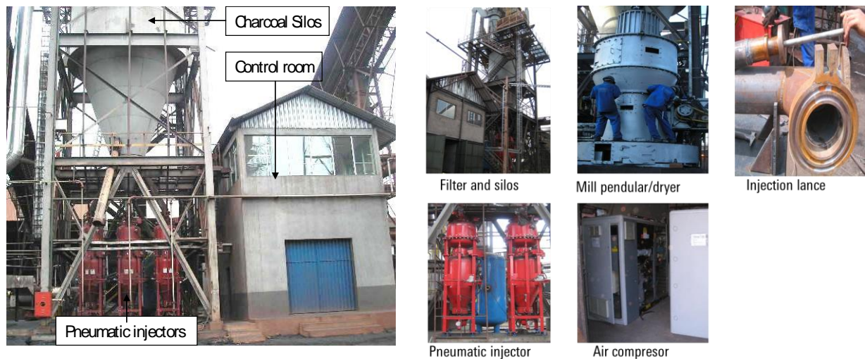
Figure 38. View of the Bio-PCI installation at Gusa Nordeste Source Nascimento et al. (2007)
