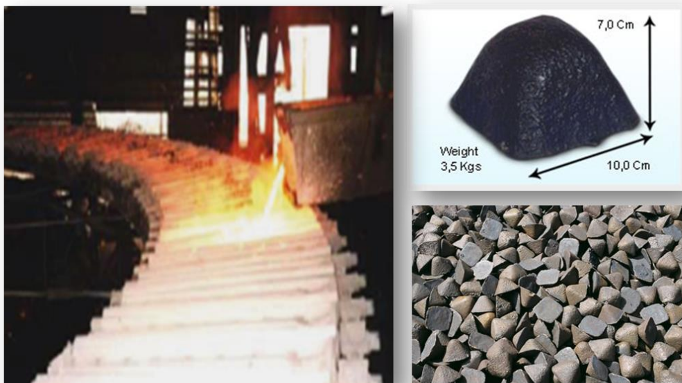
Figure 30. Charcoal- hot metal: ingot casting (left), ferro gusa or pig iron (right) Source: Valladares and Scherer (2012).
