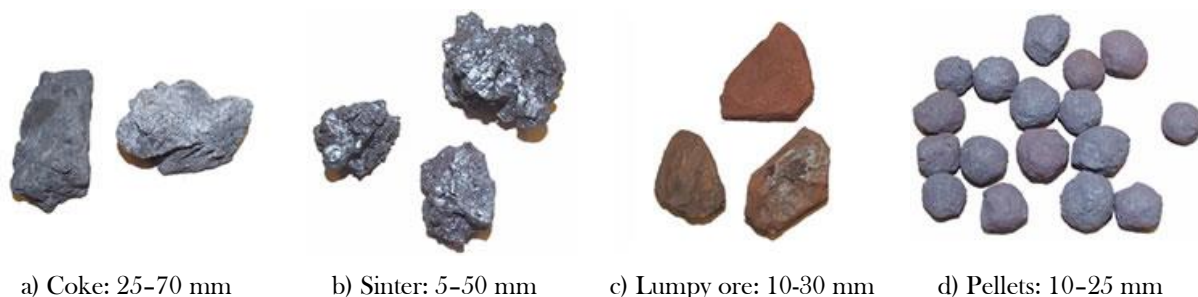
Figure 8. Main raw materials charged to the blast furnace (common size)
