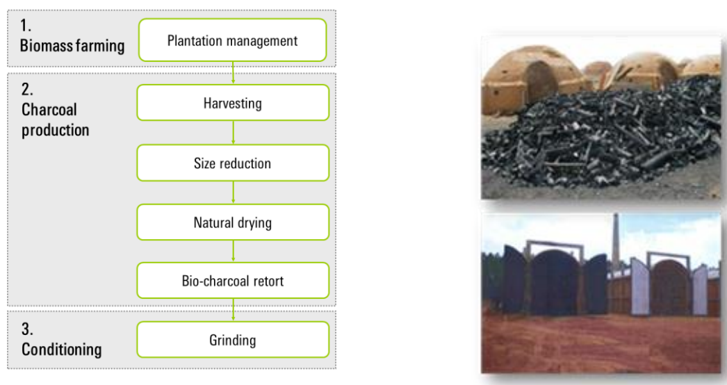
Figure 21. Unit processes of charcoal-making (left), beehive kiln (right top) and retort (right bottom)
