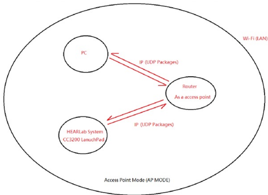
Figure 3.1: Networking topology in the HEARLab System
