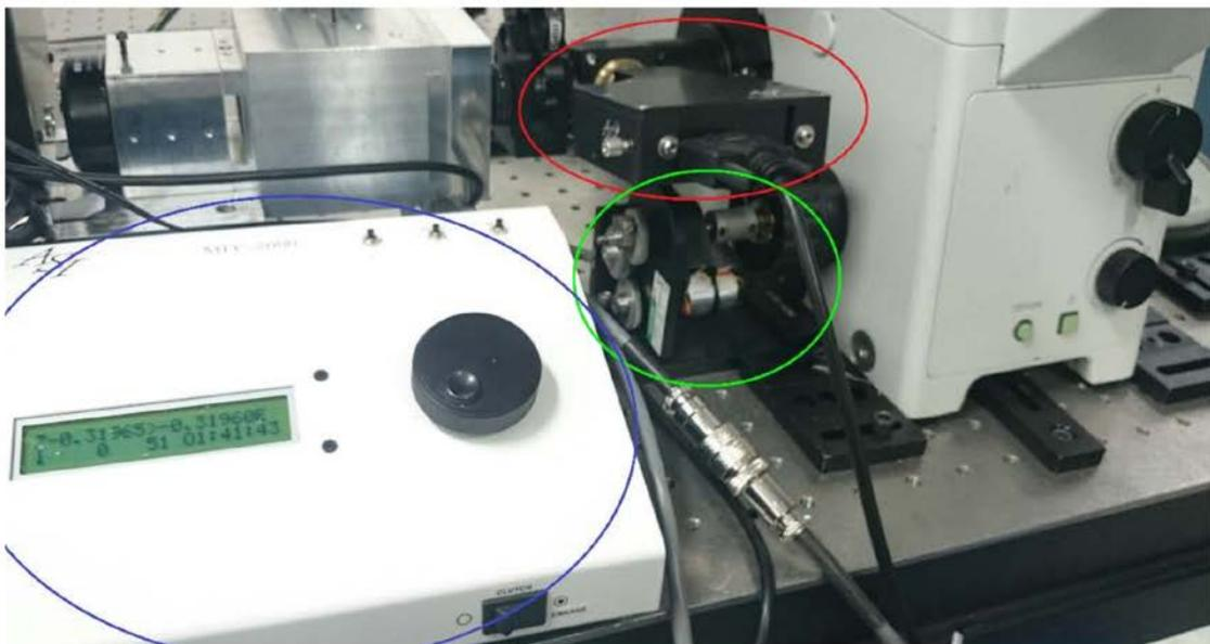
**Figure S3.** The autofocus system attached to the microscope. Red circle – feedback unit; green circle – Z-drive; blue circle – controller.
