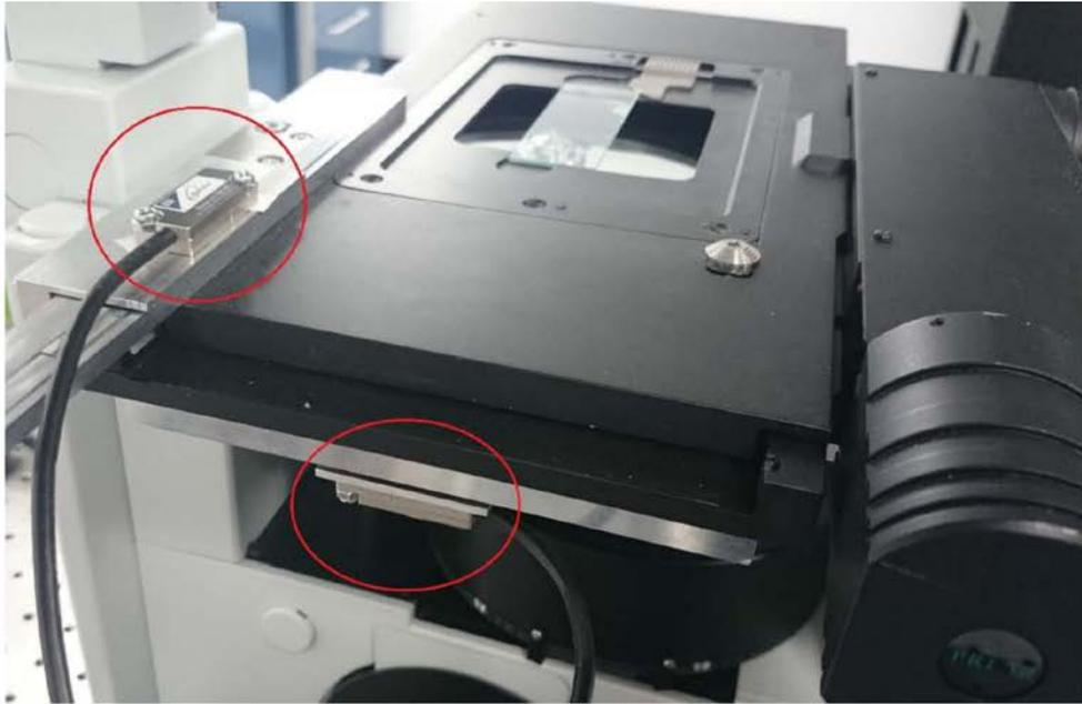
**Figure S2.** The linear encoders (circled in red) attached to the motorized stage.
