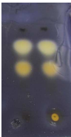
Figure 2.6.3: A simple TLC bioautography assay.
