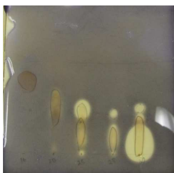
Figure 3.3.9: TLC bioautography (method 4). The bacteria grew evenly all over the plate and the clear area indicates no bacterial growth due to the presence of antibacterial compounds.
