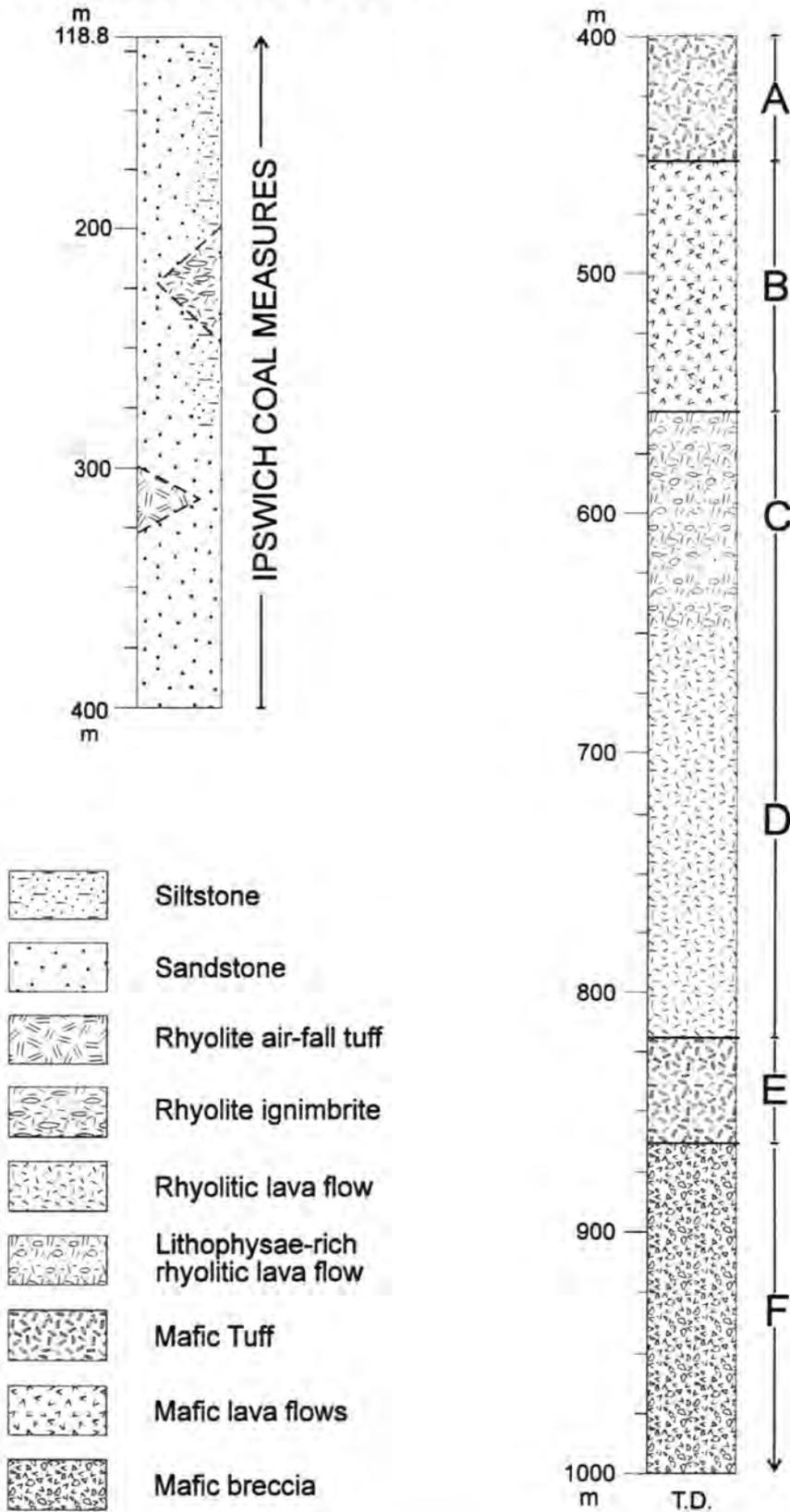
Figure 4.11 Drill log of APS Matjara No.1 (offshore southeast of Moreton Island), reinterpreted from Crook and Hoyling (1968).
