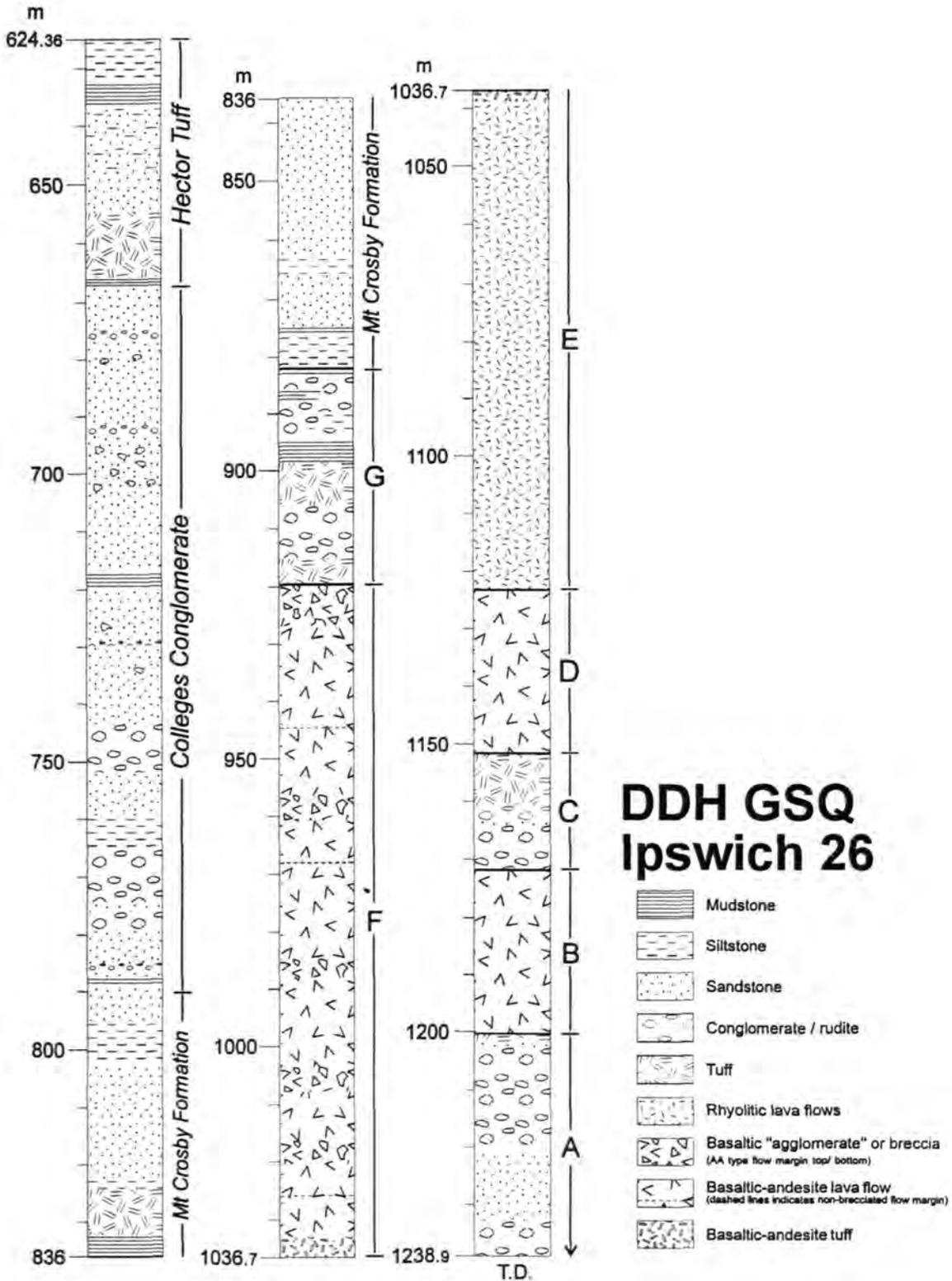
Figure 4.9 Drill log of GSQ Ipswich 26 based on Almond (1982) and reinterpretation of drill core.
