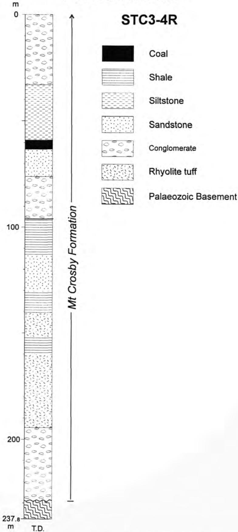
Figure 4.4 Drill log of STC 3-4R, through the Mount Crosby Formation near Pine Mountain (after Cranfield *et al.*, 1976).
