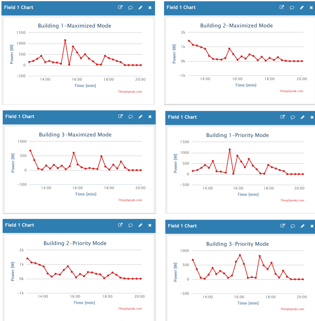
FIGURE 3.7: Graphical interface of the ThingSpeak channel representing excess solar generation of each building in each operational mode.
