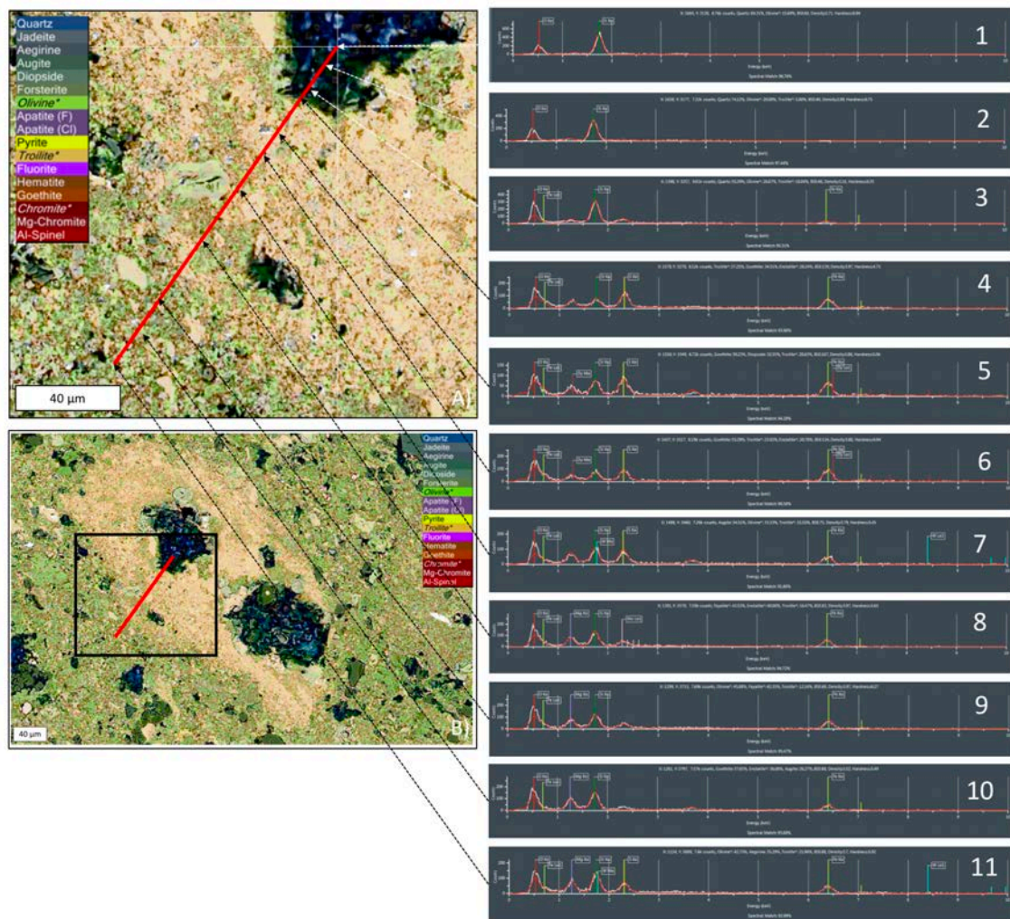
Figure 4.11 - Feature 1 - reaction rim around two \text{SiO}_2 grains, seen in Murchison ROI 2. The transect is indicated with the red line and at each point, shown with the arrows a spectrum was taken (right). The scale and key are provided for each NanoMin map.
