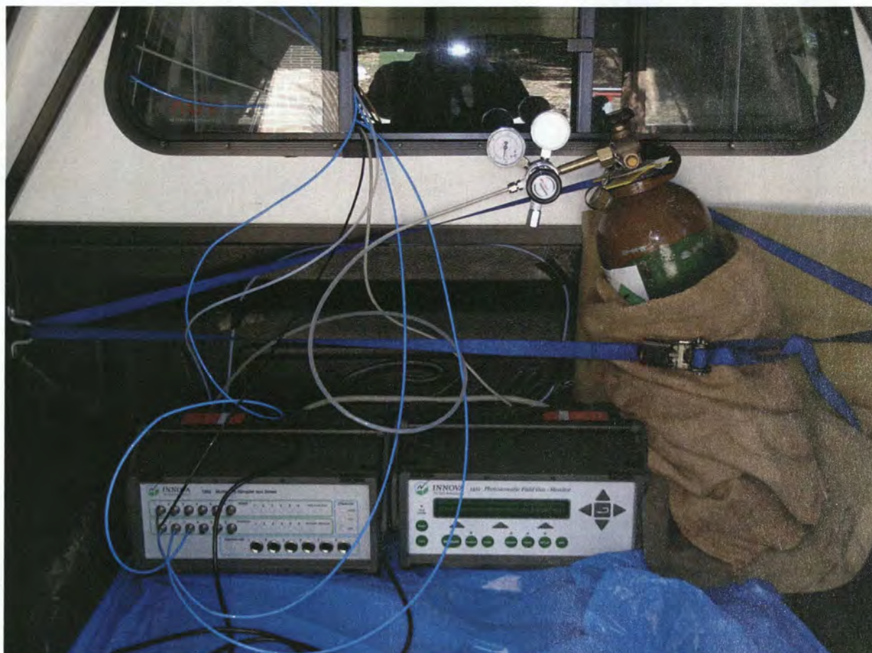
Figure A-9. Innova 1303 sampler/doser (left) and 1412 photoacoustic gas monitor (centre) next to the SF 6 cylinder in the cargo tray of the 2005 Toyota HiLux.
