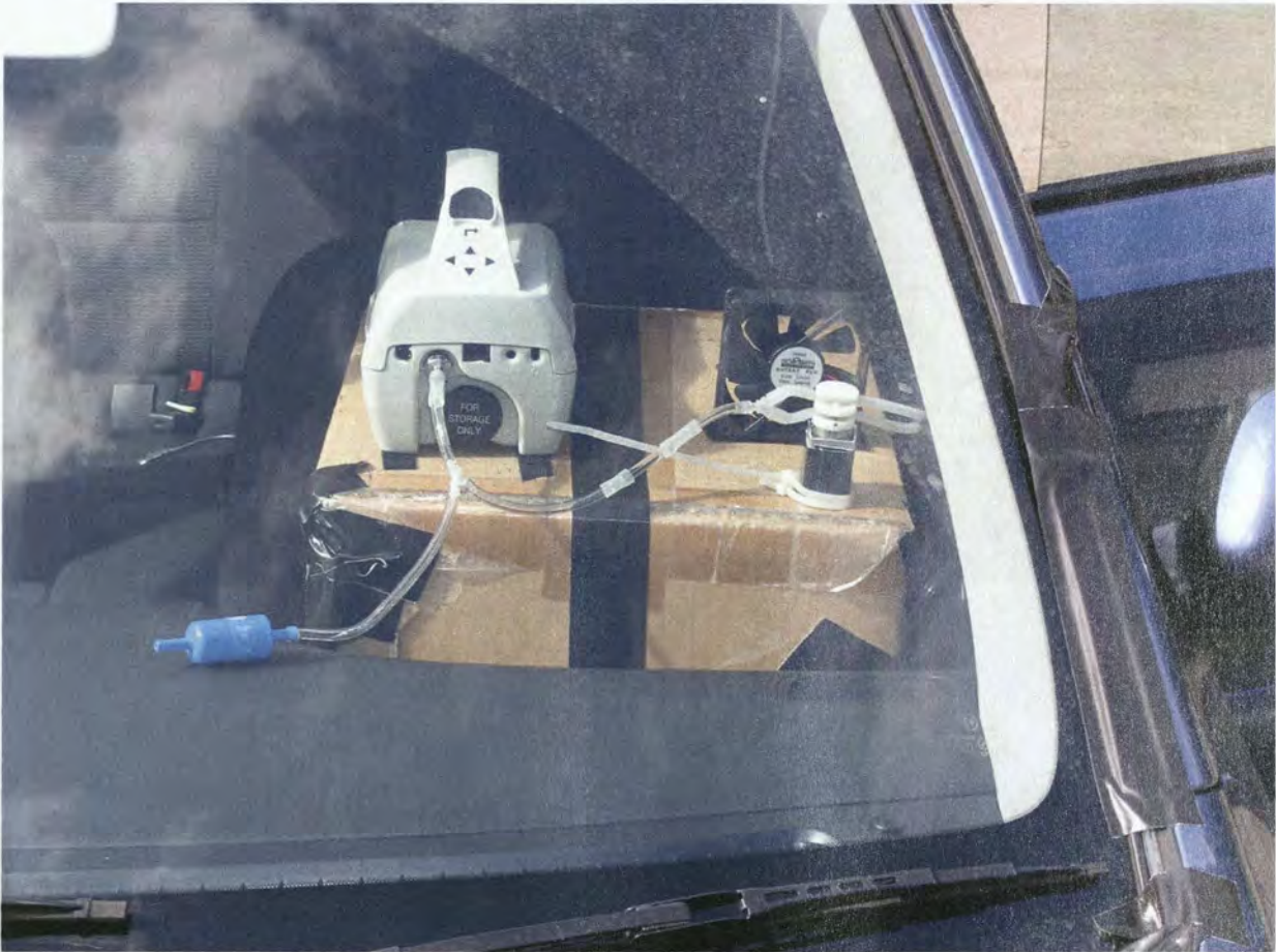
Figure A-17. TSI 3007 CPC (affixed to cardboard by Velcro) with dilution system, sampling point switching valve and small fan seen from through the front windscreen of the 2007 Subaru Outback.
