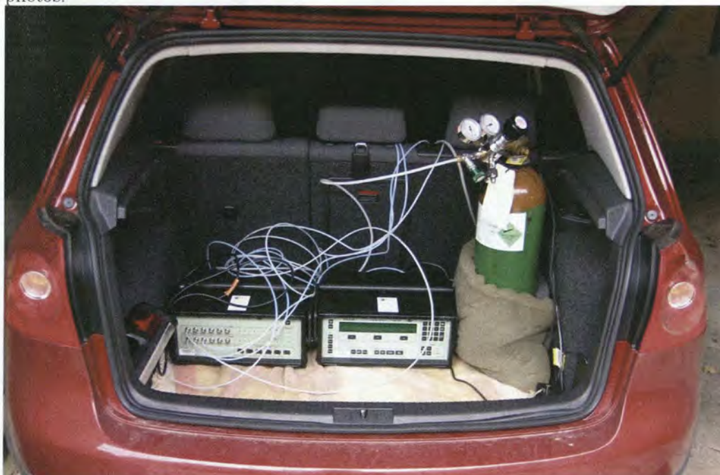
Figure A-8. The same experimental instruments described in figure A-7 can be seen here in the boot of the 2005 Volkswagen Golf, in addition to the SF 6 cylinder (prior to being secured). The batteries and power inverter were fitted after this photo was taken.
