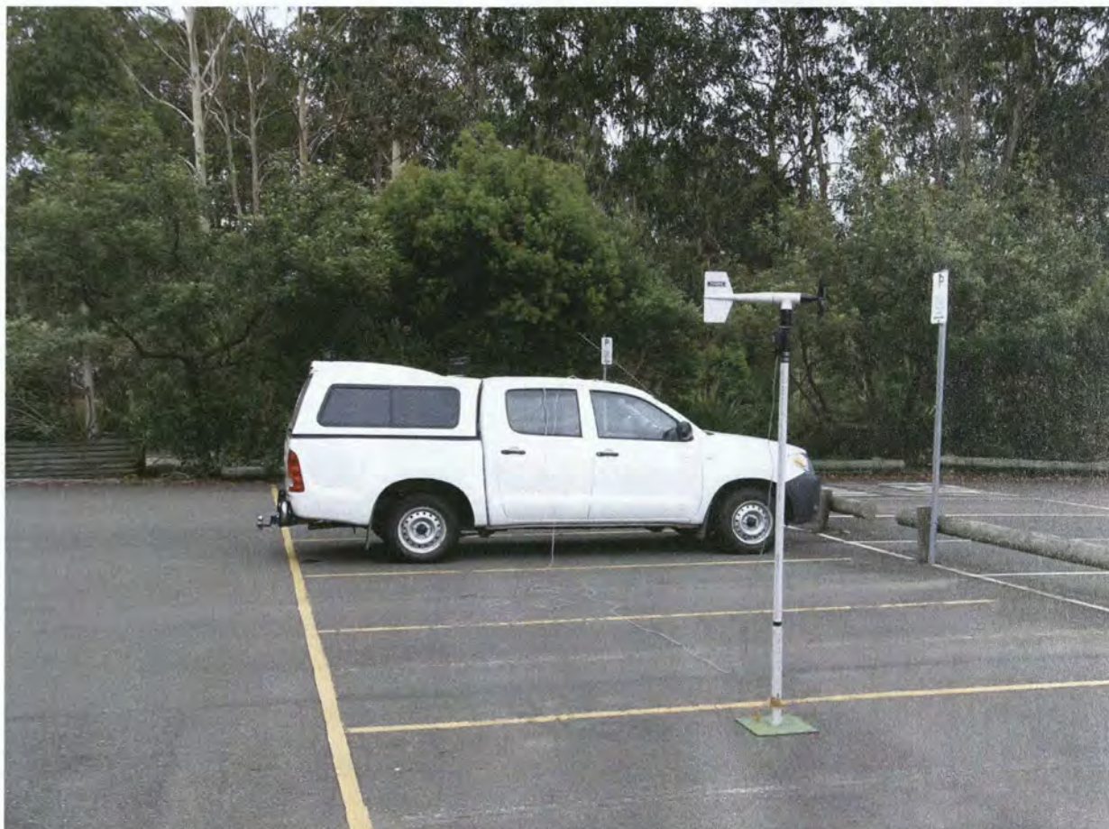
Figure A-13. 2005 Toyota HiLux prior to a stationary infiltration measurement; RM Young 05103 wind speed and direction monitor in the foreground.
