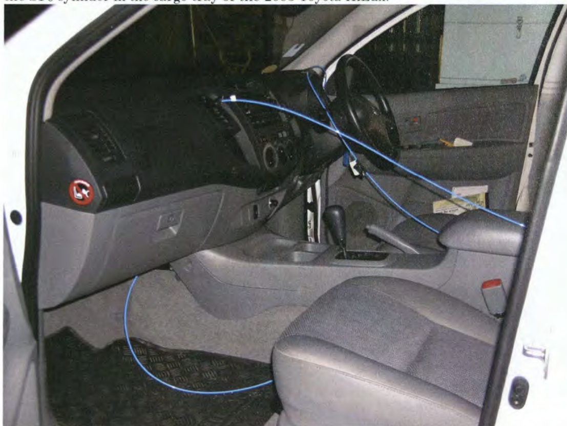
Figure A-10. Sampling points for a constant tracer gas emission measurement inside the 2005 Toyota HiLux.
