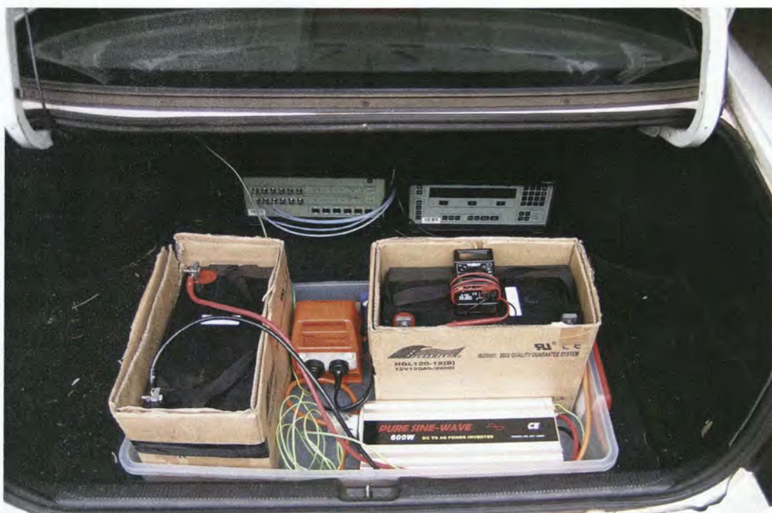
Figure A-7. Experimental equipment and power supply set up in the boot of the 1998 Mitsubishi Magna prior to an early (Jan 2006) ventilation measurement. The Brül & Kjær 1303 sampler/doser (rear left) and 1302 photacoustic gas monitor (rear right) can be seen, along with the two 120 Ah absorbed glass mat deep cycle batteries and pure sine-wave inverter used to produce the required 240 volt power. The SF 6 cylinder cannot be seen in this figure; in order to transport it in a safe (i.e. upright) manner, it was secured in the rear of passenger compartment. Note that foam padding was used to protect the instruments, but was removed for clarity prior to taking photos.
