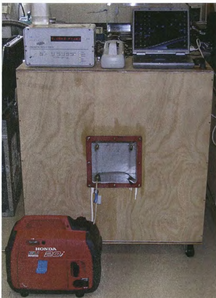
Figure A-15. Four stroke petrol generator, test chamber, TSI 3022A CPC (top left), TSI 3007 CPC (top centre) and laptop computer set up prior to laboratory test of dilution system performance.
