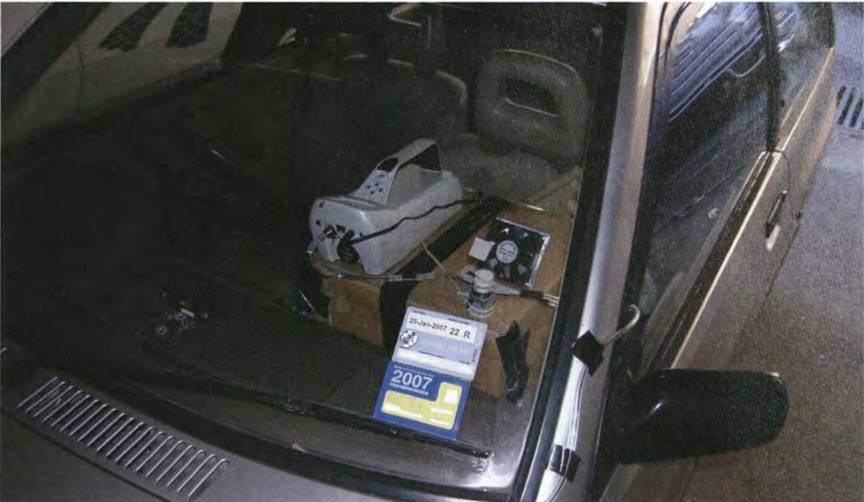
Figure A-18. As above, except the vehicle is the 1989 Mazda 121. The external (i.e. on-road) sampling line can be seen extending from a small hole made through a thick tape seal placed over the front passenger side window
