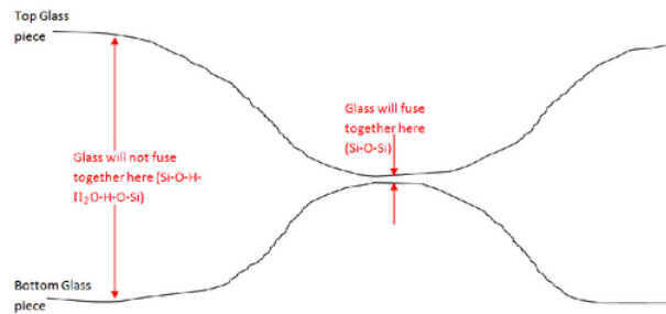
Figure 2.15: The fusion bond (Si-O-Si) will form at peaks on the glass surface where the surfaces are sufficiently close together.
