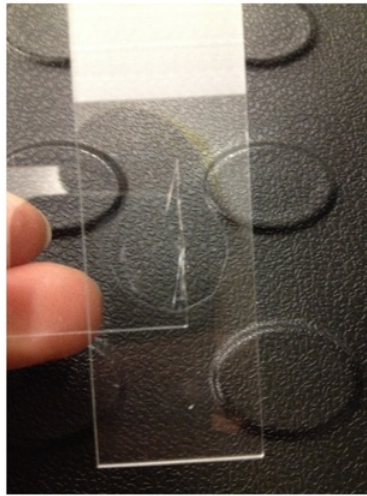
Figure 3.5: Breakage of sample following peeling test attempt on a glued sample.
