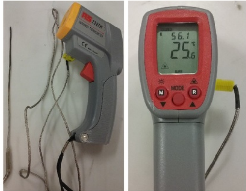
Figure 6.9: Thermometer and thermocouple attachment
