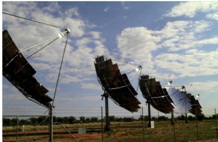
Figure 2.2: Parabolic dish collectors with central receivers [8]
