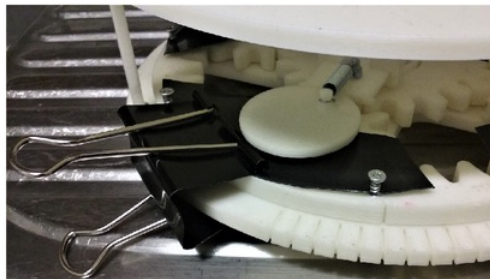
Figure 6.10: Mechanism fixed in notch position using clips
