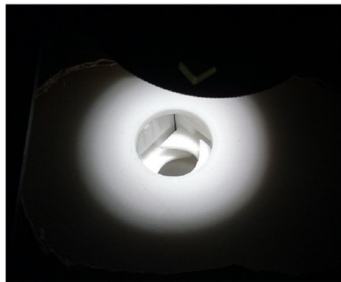
Figure 6.12: Solar simulator light shining onto receiver below aperture
