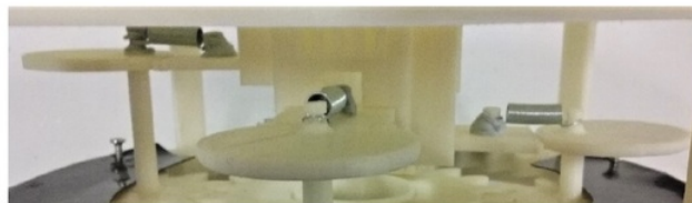
Figure 4.5: Springs to return followers to resting position when cams move away
