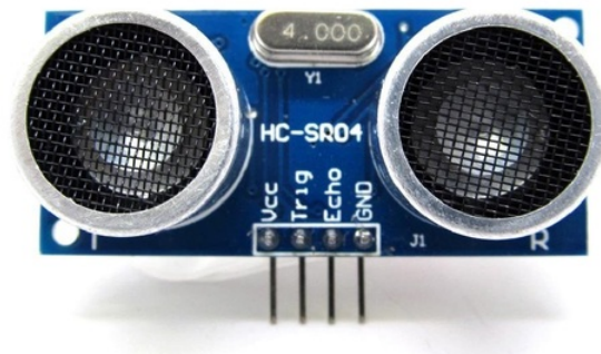
Figure 2.13: HC-SR04 Ultrasonic sensor [10]
