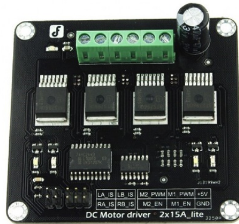
Figure 2.12: DC Motor Driver Lite from DFRobot [9]
