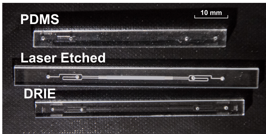
Figure 3.5: The three devices that were created by different fabrication processes. The ports of all three devices are visible but the channel visibility varies with surface roughness. The inability to see the channels of the PDMS and DRIE devices indicates a smoother surface. The channel of the laser etched piece appears frosted due to the rough finish produced by the laser etching process.
