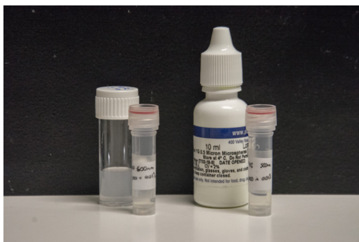
Figure 4.1: The nanomaterial dilutions that were processed in the laser scattering experiment placed in front of the larger stock containers. The bulk ND samples are on the left and the fluorescent bead samples are on the right.
