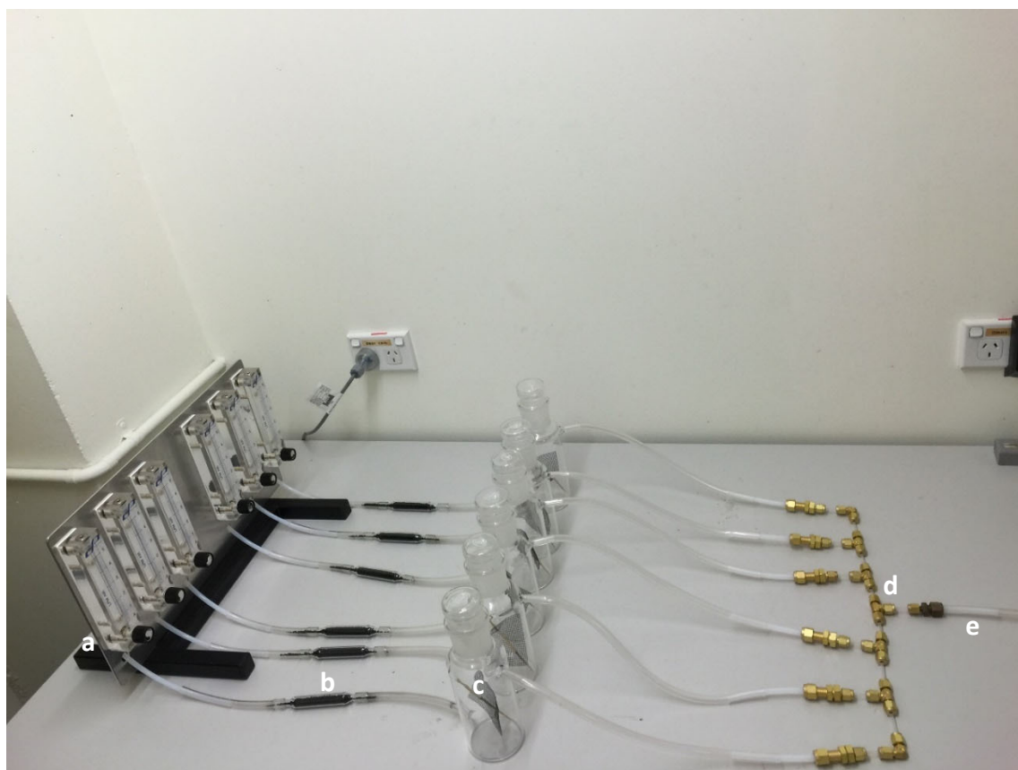
Figure 1. Setup of air trapping system for collecting volatiles from false garden mantids. Flowmeter (a), active charcoal filter (b), container for mantids (c), air merge (d) and tenax filters (e).
