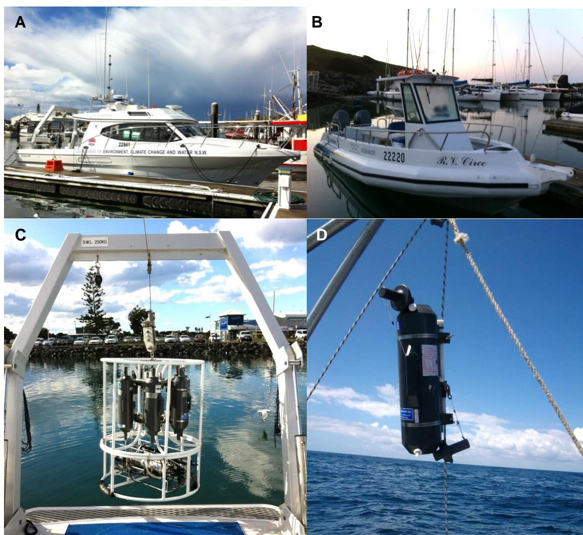
Figure 3. Research Vessels and sampling equipment. A) RV Bombora provided by the New South Wales Office of Environment and Heritage, Sydney, and B) RV Circe provided by the National Marine Science Centre, Coffs Harbour, to undertake the field campaigns in the Coffs Harbour region. C) A-frame and sampling rosette including Niskin bottles and CTD on RV Bombora . D) Niskin bottle manually attached to a rope on RV Circe .
