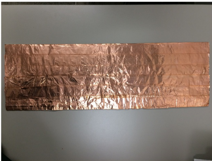
Figure 3.6: The bottom of the prototype of the multi-array antenna design. This acted as the ground plane.
