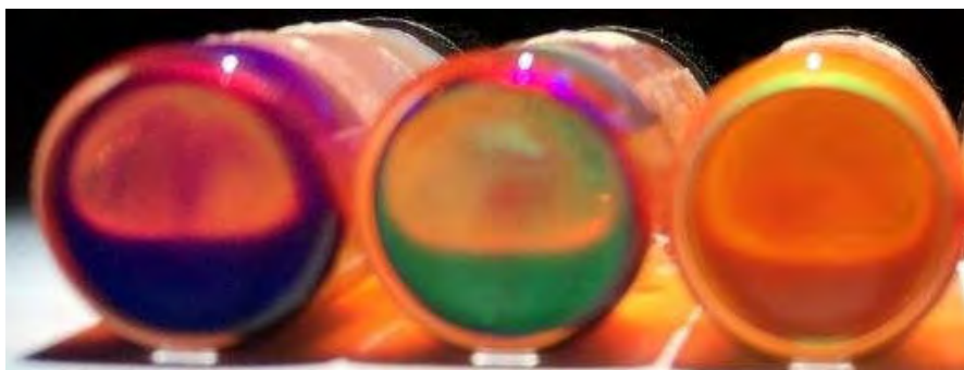
Figure 57 RGB colour cells obtained from an azo-carrying TBA in an achiral LC host (7CB)
