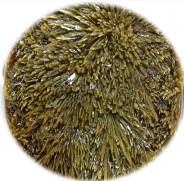
Figure 53 Images of the produced crystals of TBAs
