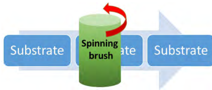
Figure 6 Brushing method for mechanical alignments
