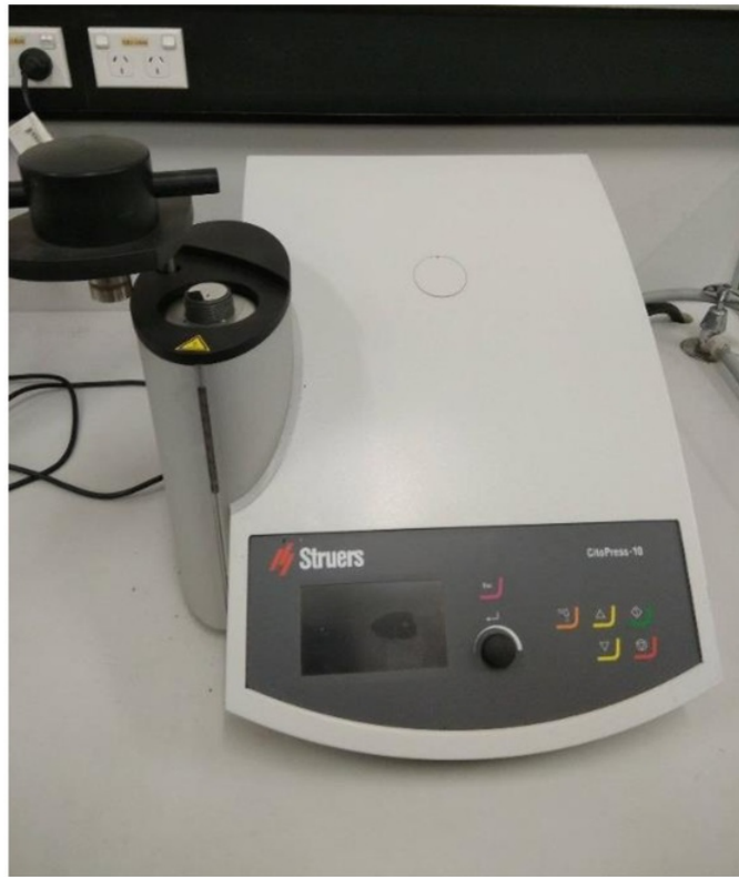
Figure 12: The Struers Citopress – 10 sample preparation apparatus
