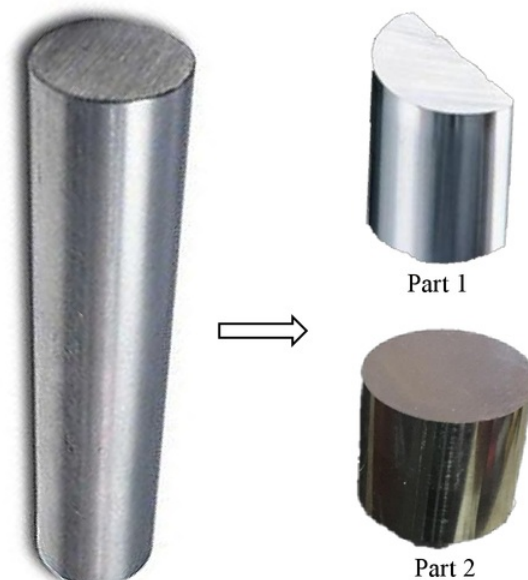
Figure 7: Reference 316L stainless steel rod and the corresponding cuts
