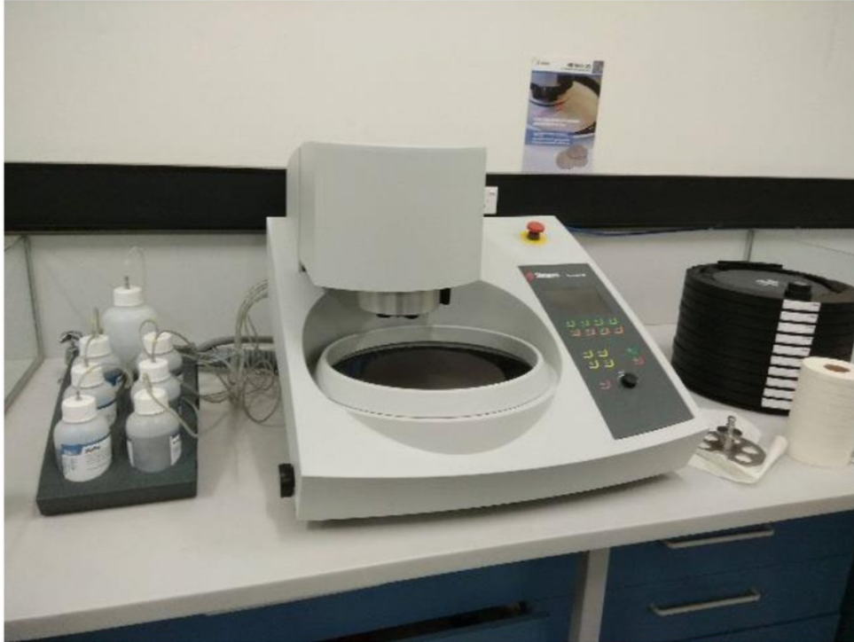
Figure 14: Struers Tegramin - 25 sample polishing apparatus
