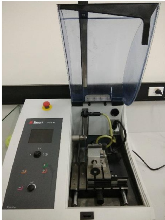
Figure 11: Figure 10: Struers Secotom – 50 sample preparation apparatus
