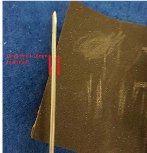
Figure 46 Polished Drawn 1.78mm Zinc 99.99% wire
