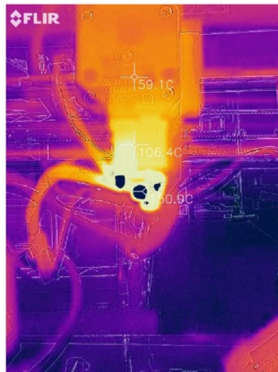
Figure 43 Initial thermal imaging of Dyze extruder system. Motor block 59.1°C nozzle 150.9°C
