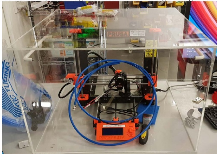
Figure 37 Final assembly of printer system. Printer with Dyze head, filament, gas tube and chamber.
