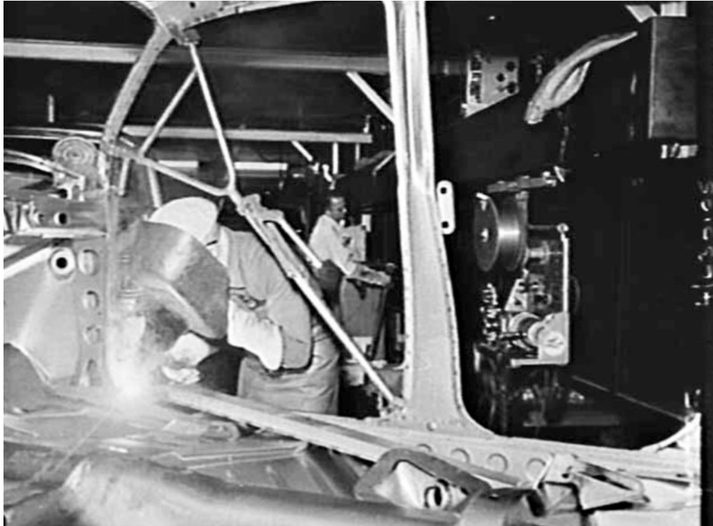
Figure 7.7: Don McPhedran, 'Motor body builders use CIG welding equipment to weld the new EJ Holden, Pagewood'.
