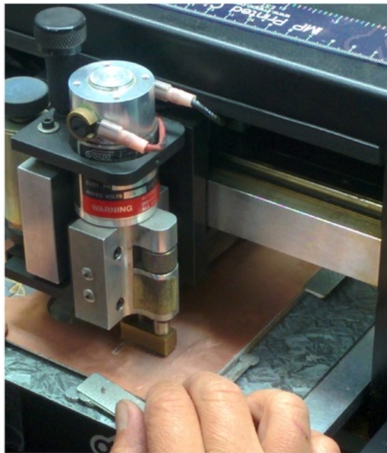
Figure 5.7: The Quick Circuit routing and milling machine Fabricating the circuit
