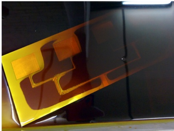
Figure 5.3: Chemical Etching of Antennas
