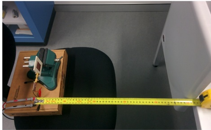
Figure 6.11: Experimental setup for Rectenna System-1 testing in the laboratory
