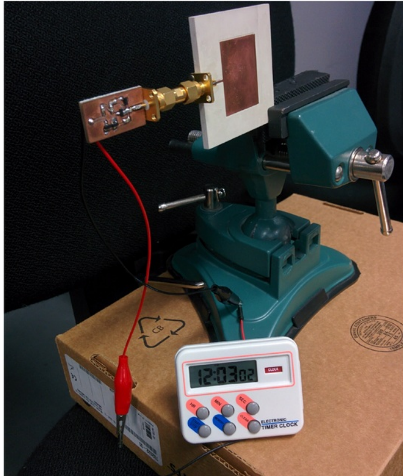
Figure 6.16: Rectenna System 1 Powering a digital clock timer
