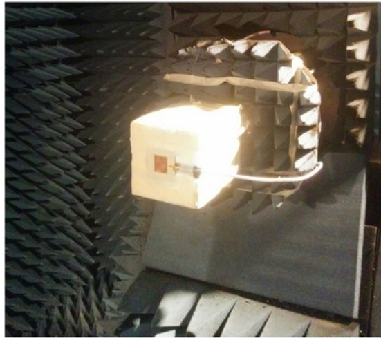
Figure 6.3: Experimental setup in anechoic chamber with microstrip patch antenna
