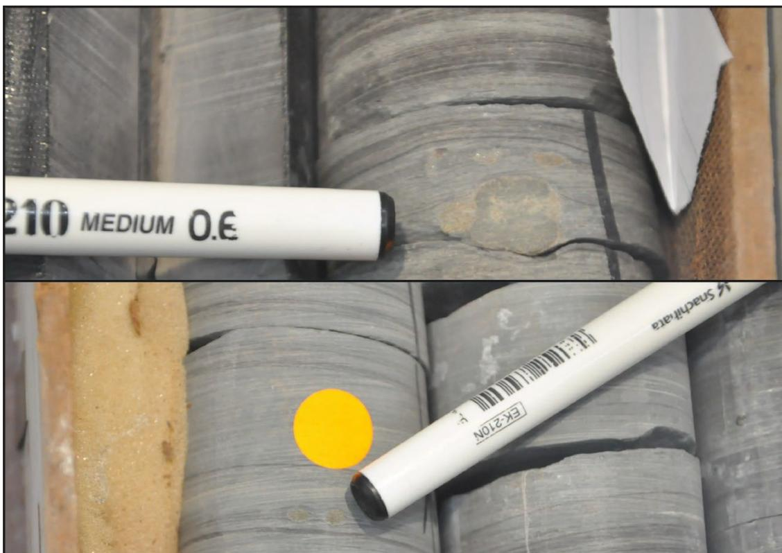
*Figure 3: Pyrite nodules at ~ 110m in Urapunga – 4. Top; nodule is ~1cm in diameter, and shows sediment draping textures. Bottom; nodules are < 0.5cm, and show draping textures.*
