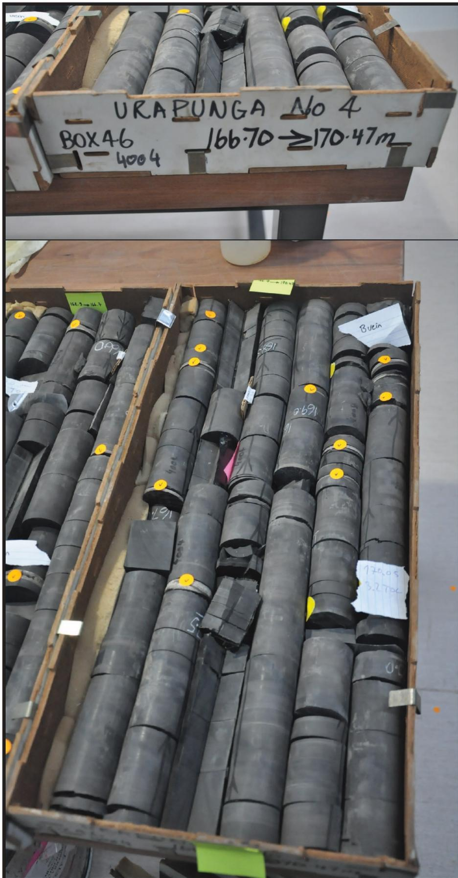
Figure 4: Orange stickers indicate where veins are observed within the Urapunga 4 core between 166.7m and 170.47m
