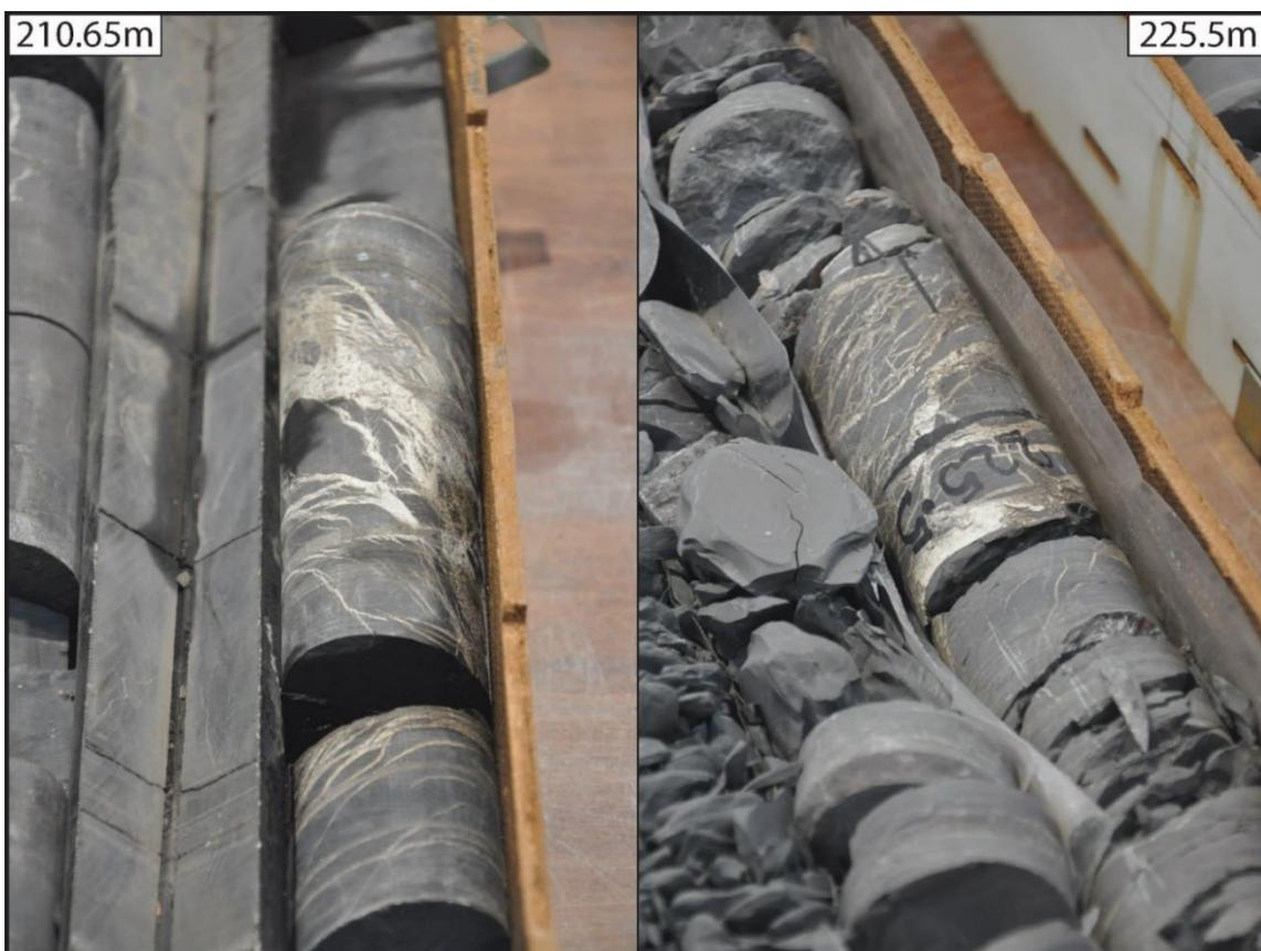
Figure 2: Examples of breccias within Urapunga - 4 core. Breccias exhibit crackle break textures, and show evidence of multiple cross cutting veins.
