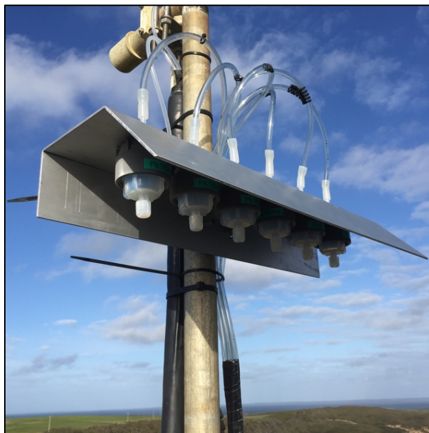
Figure 2.5 Ambient reactive mercury filter deployment setup at Cape Grim Baseline Air Pollution Station, improved upon from the University of Nevada Reno Reactive Mercury System (photo by author).
