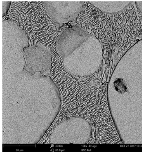
Figure 4.8: Microstructure of Zn-0.8Mg heat-treat at 300°C
