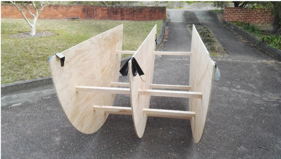
Figure C.3: The result when the three pieces were combined. Two more cross beams were later added closer to the top of the reflector to increase sturdiness.
