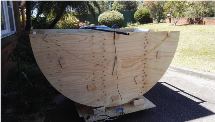
Figure 5.3: Reflector and tracking system combined to form the final system.
